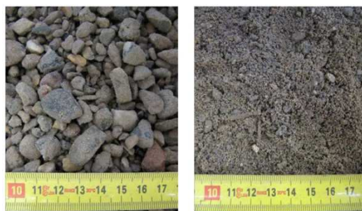
Figure 5. Products from crushed concrete by ADR: Coarse (left) and Fine (right).
