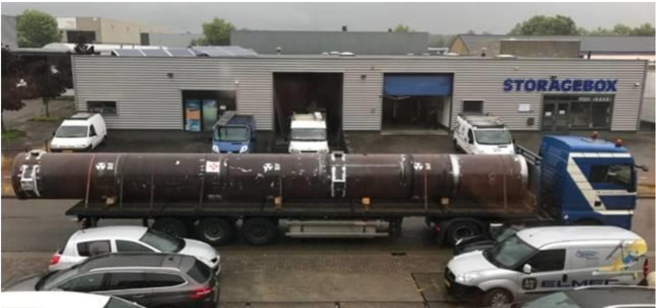
Figure 8: 1.6 m diameter steel construction used for environmental loading tests to obtain the settling behavior of the DSJ connection
