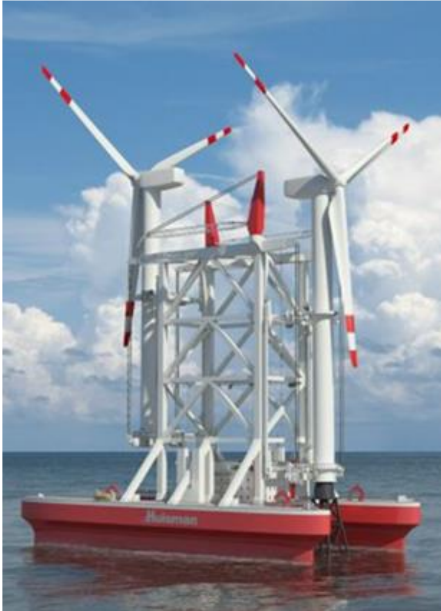
Figure F. 3: Huisman Wind Turbine Shuttle concept transporting and installing two wind turbines.
