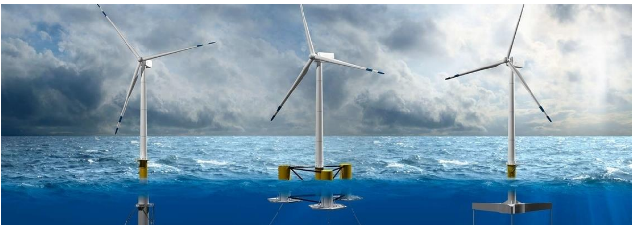
Figure 5: Three main floating wind concepts (source: NREL, illustration by Josh Bauer)
