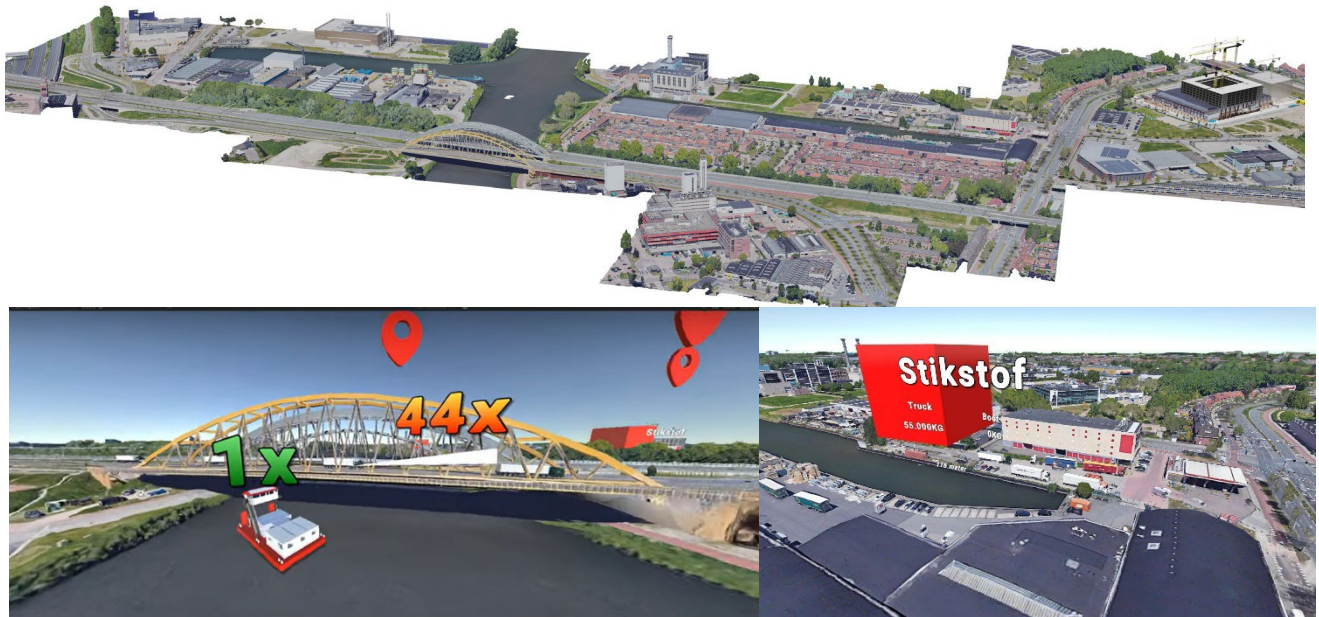
Figure 5. Modelling the last mile of supply chain to construction site, including traffic analysis, and modal shift scenario comparison when using ships instead of trucks for construction transport (Stikstof is Dutch for NOx) (Case Utrecht)
