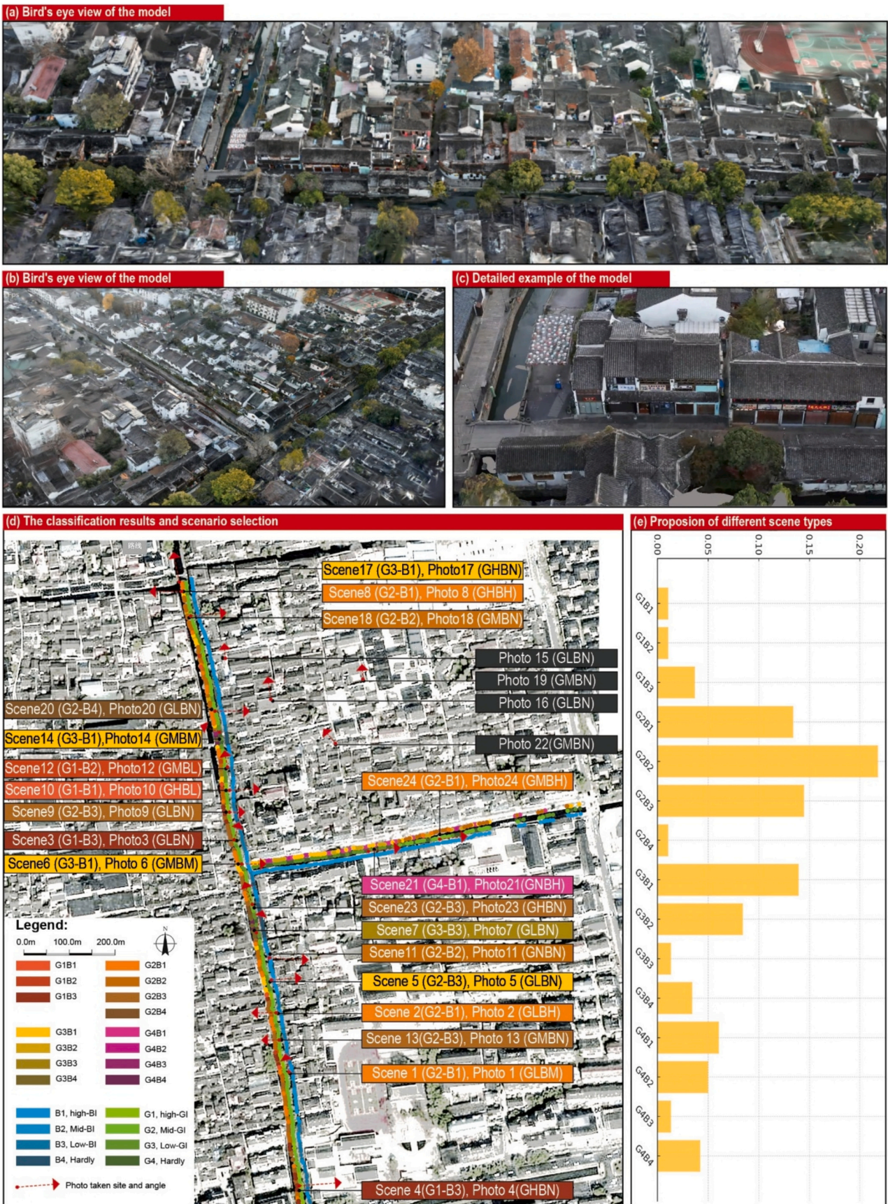
Fig. 3. (a)-(c): Visualization and modeling results; (d)-(e) Scene type classification based on BI and GI exposure.
