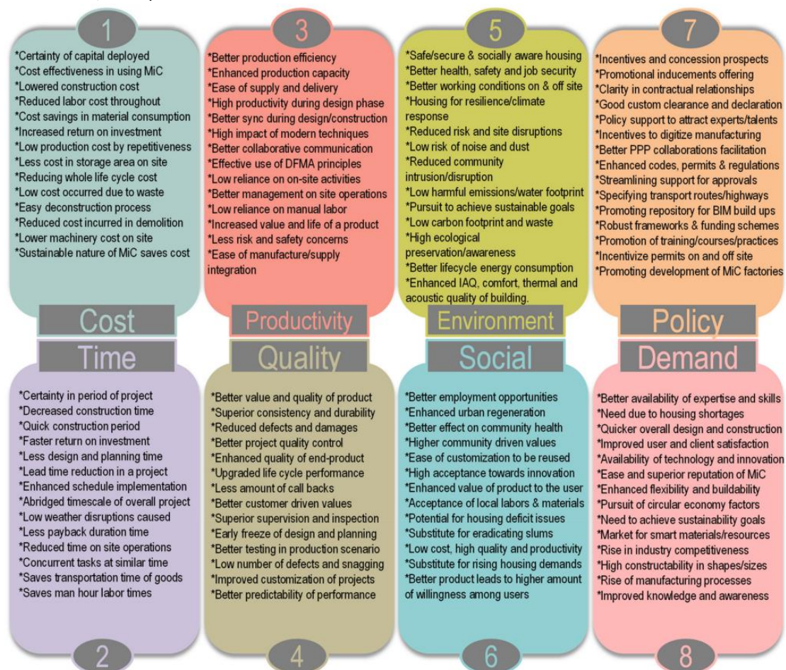
Figure 1: 111 Drivers towards modular integrated construction (Khan et al, 2011)
