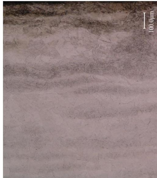
Figure 31: Solid dilatometric sample 5 K/s. The sample edge is at the right.
