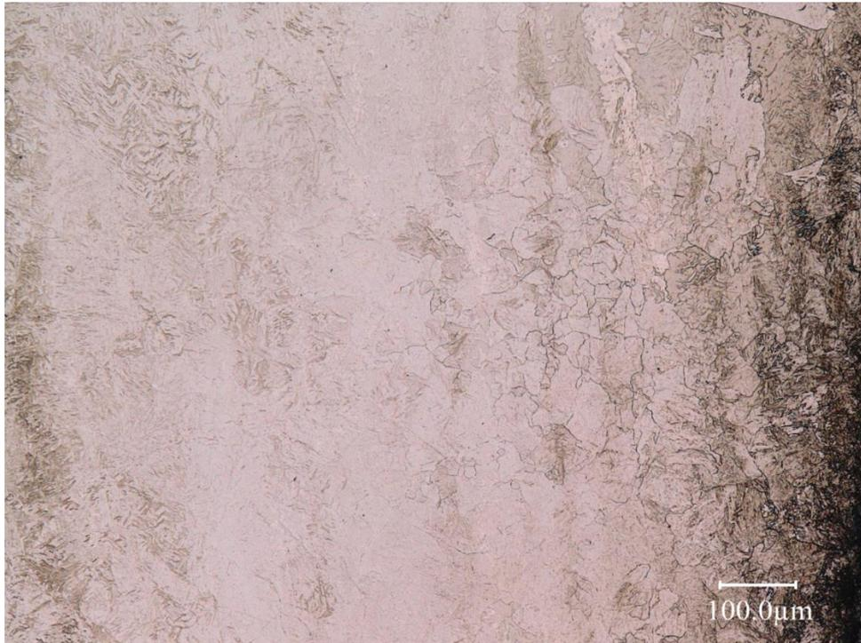
Figure 34: Hollow dilatometry sample, 500 K/s. The sample edges is at the right.
