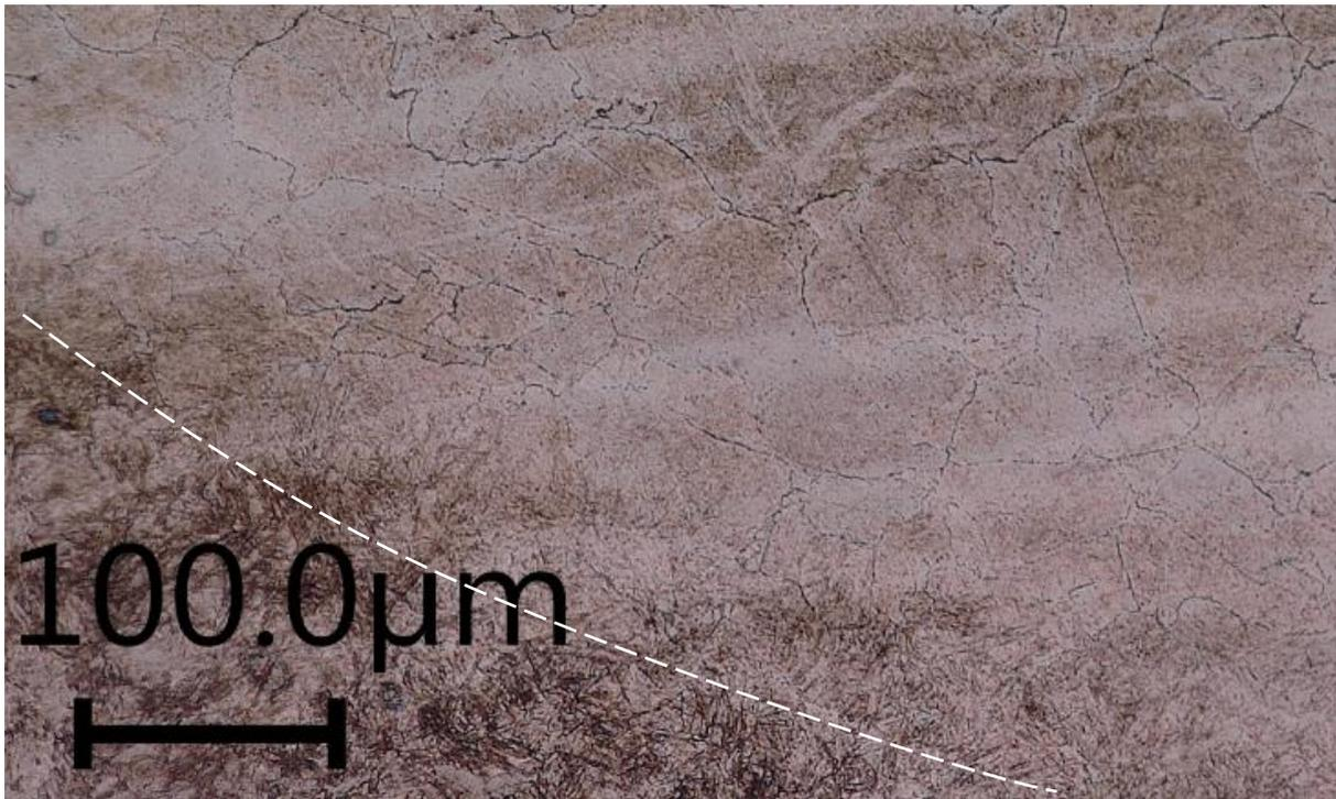
Figure 51: Deep zone, near the interface with martensitic parent structure (Dashed white line).
