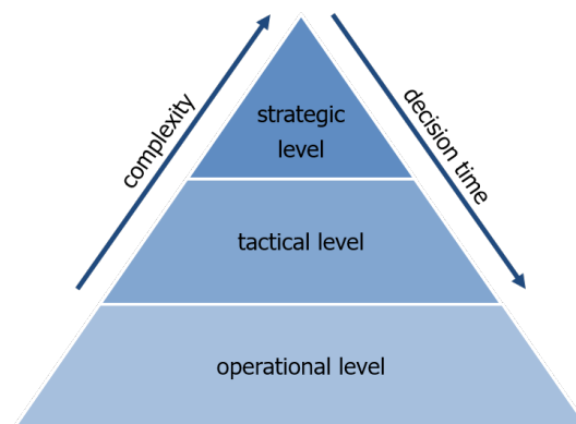
Figure 4.20: Three driving task levels and complexity and decision time (translated from [52])
