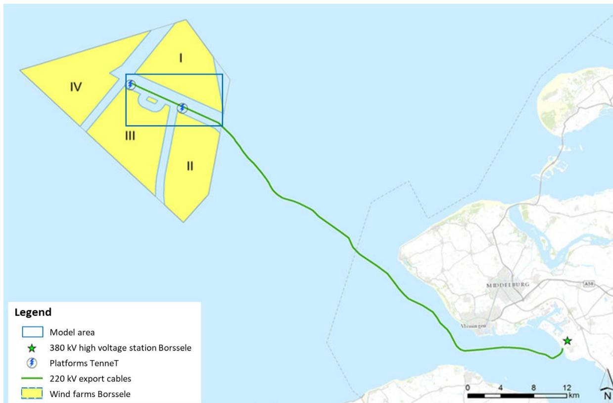
Figure 1.2: Route of the export cables (green) between windfarms Borssele I + II and the main land (modified, based on Provinciale Zeeuwse Courant (2019)). The case study area is indicated by the blue box.
