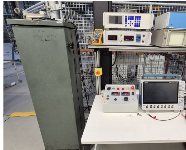
(b) The control side of the experiment, showing the autotransformer, the oscilloscope and the control devices
