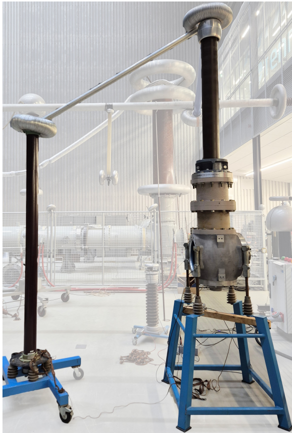
(a) The test compartment connected to a coupling capacitor
