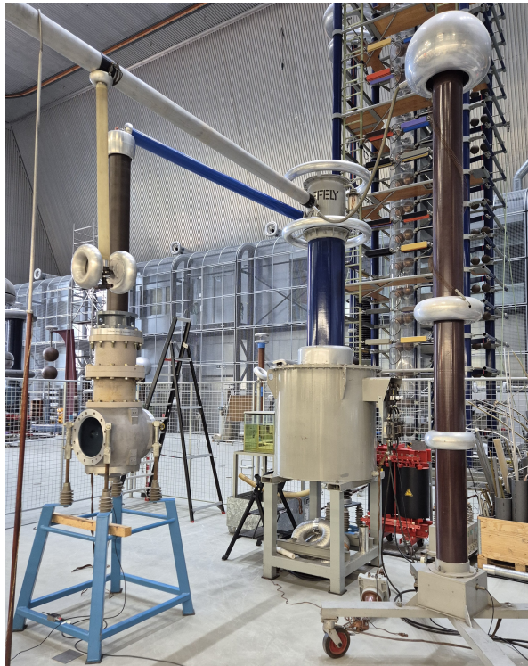
Figure 5.5: Capacitive voltage divider and the HV transformer connected to the test compartment through the (blue) blocking resistor
