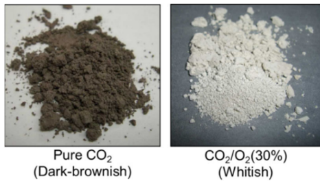
Figure 2.1: Solid by-products after arcing in pure CO 2 gas and CO 2 /O 2 gas mixture after 1,900 kJ accumulative interruptions [2]
