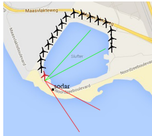
Figure 87: The favorable and unfavorable wind directions illustrated on a map. Green sector is favorable ( 42^\circ - 62^\circ ), the red sector is unfavorable ( 118^\circ - 146^\circ )
