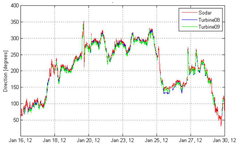
Figure 22: Nacelle direction of turbines 8 and 9 (corrected by 53^\circ ) compared to wind direction as measured by the Sodar at 65m through time series plot
