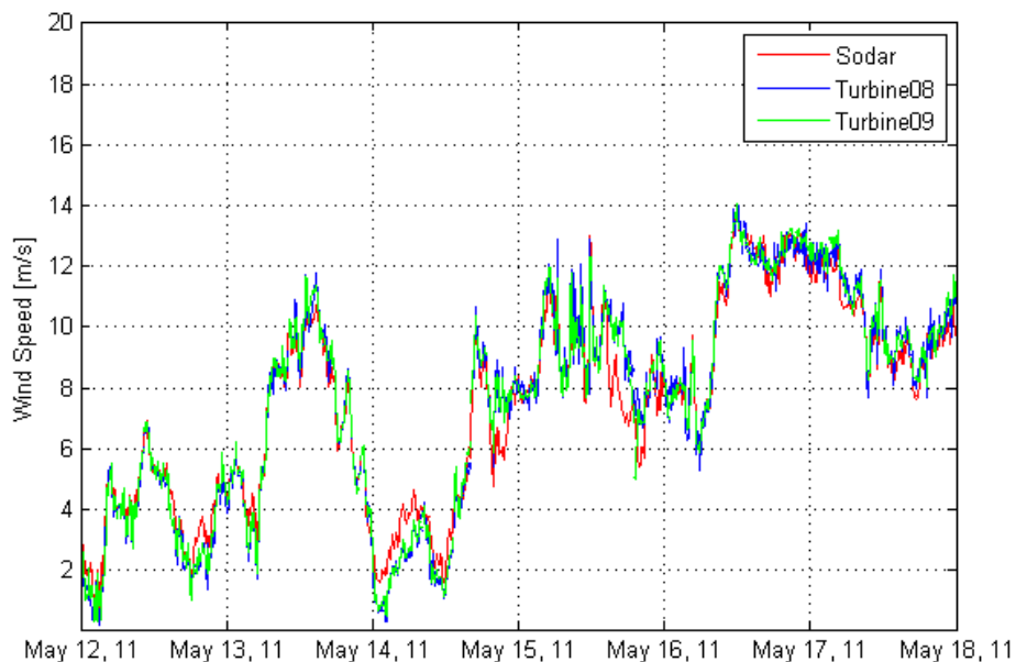
Figure 15: Comparison of wind speed as measured by the sodar and nacelle cup anemometer of turbine 8 and 9
