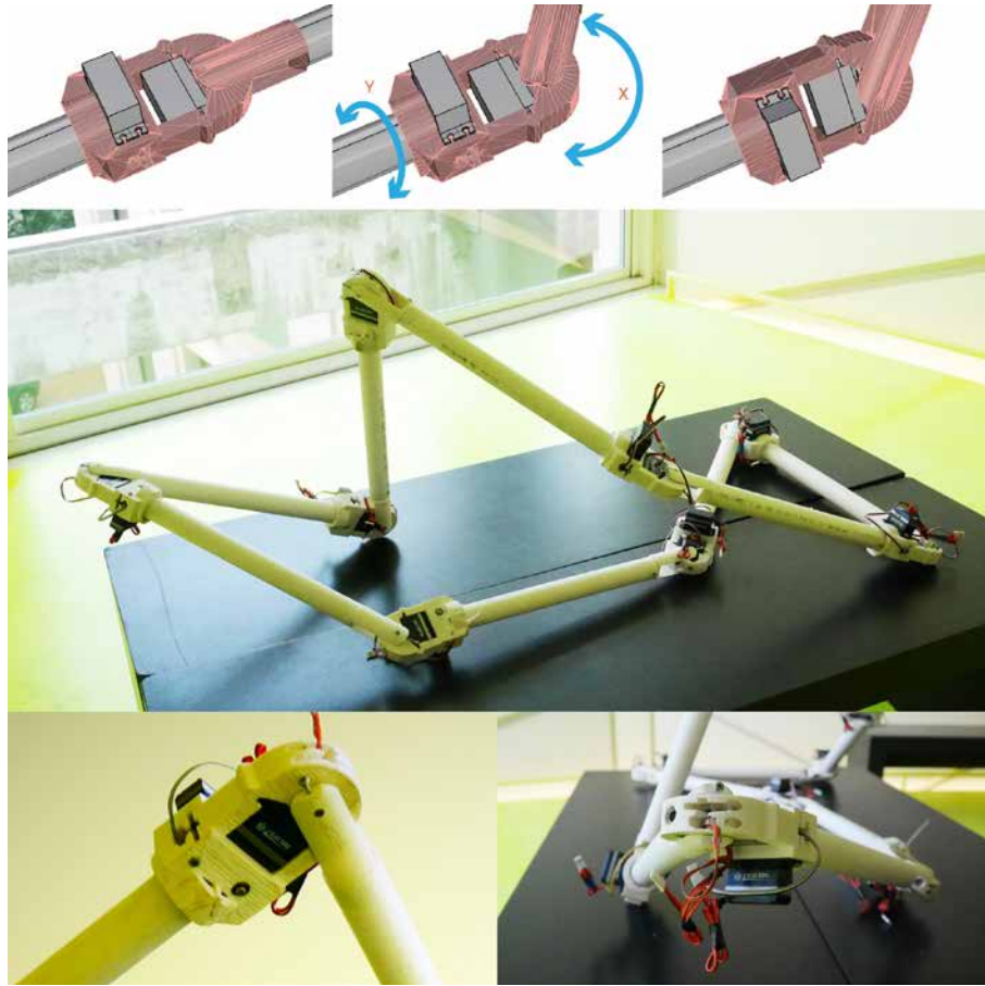
FIGURE 6.25 Images exhibiting the simulations, the prototype scale model of the HyperLoop pavilion, and a closer look at the joint design and prototype.
