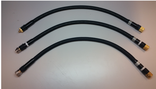
Figure 2.13: Examples of phase-stable VNA test-port cables used at the VSL RF laboratory.
