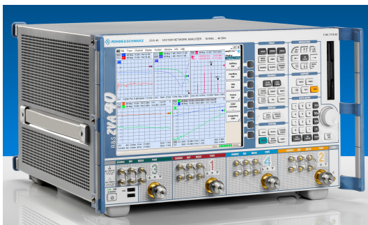
Figure 2.9: A photograph of a four-port ZVA40 Vector Network Analyzer from Rohde & Schwarz.
