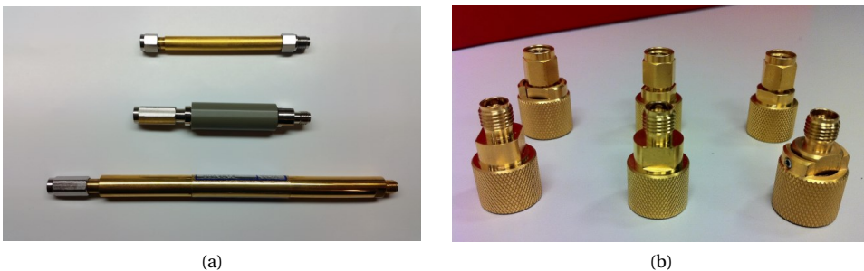
Figure 2.19: (a) Metrology grade coaxial air-dielectric transmission line standards. (b) An overview of metrology grade coaxial SOL calibration kit.
