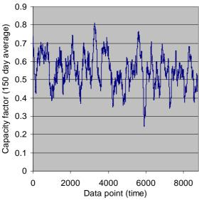
Figure 11: 150 day walking average capacity factor versus time.
