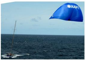
Figure 12: Cloth kite replacing sails of a sailing boat [7]
