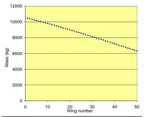
Figure 8: 100 MW laddermill wings mass
