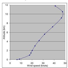
Figure 1: Average wind over the Netherlands versus the altitude [1]
