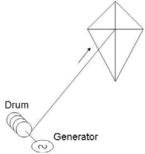
Figure 2: Simple illustration of the Laddermill principle
