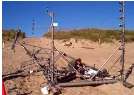
Figure 6.23 Sled used to collect the current velocity at different vertical elevations ( www.frf.usace.army.mil/sandyduck/ )
