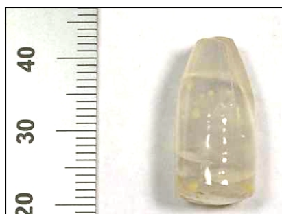
Figure 13a. Photograph of a \text{SrI}_2:\text{Eu} crystal grown at RMD with 1 cm diameter, 2.4 cm length.
