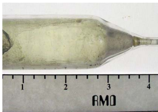
Figure 13b. Photograph of a \text{SrI}_2:\text{Eu} crystal grown at RMD with 1" diameter, \sim 2" length.
