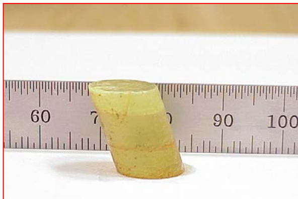
Figure 1. Photograph of a \text{LuI}_3\text{:Ce} crystal (in which its layered structure is evident) grown by Bridgman.
