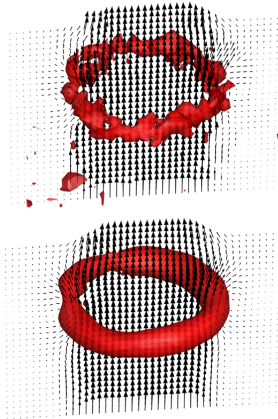
Figure 2.17 Three-dimensional velocity field measurement at the exit of a laminar jet. A vortex ring is formed at approximately one diameter downstream the nozzle exit. Iso-surface of vortex detection criterion Q (Hunt et al. 1988) in red. Cross-correlation performed without (top) and with (bottom) volume deformation.
