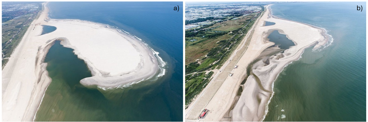
Fig. 5. Aerial photos of the Sand Engine peninsula, taken from the North in (a) July 2011 (shortly after construction) and (b) July 2012 (after the first year). Source: Rijkswaterstaat and van Houdt (2012) 76 .
