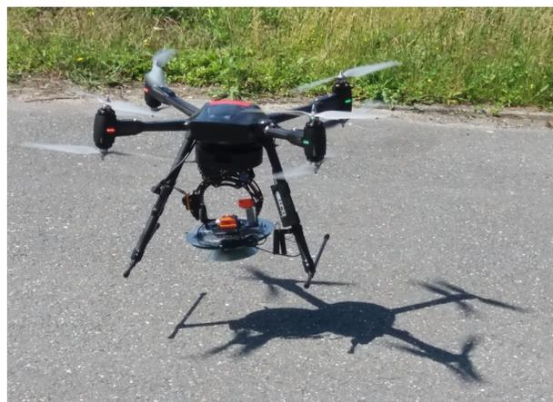
Fig. 1: The omnidirectional SAR system mounted on a drone.
