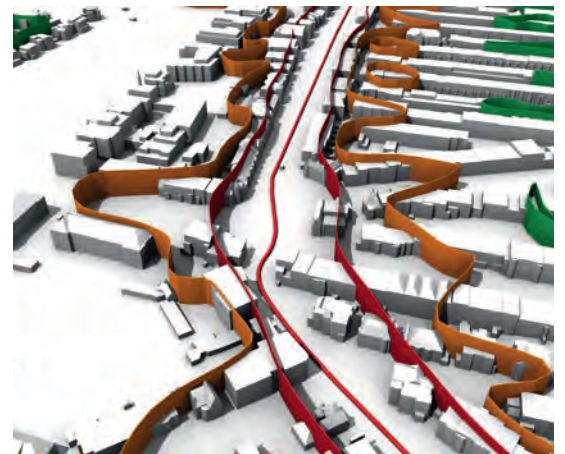
▲ Figure 2, Noise pollution by a tram line simulated with Geomilieu-DGMR on data from City of The Hague and visualised in Blender; the red, orange and green contours represent high, medium and low noise pollution, respectively.
