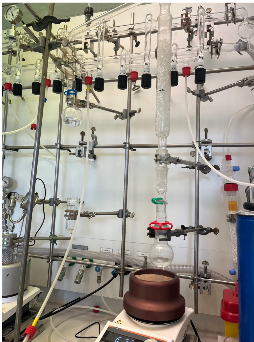
Figure 6.41: Distillation set-up with packed bed column to separate triisopropylborate from IPA.
