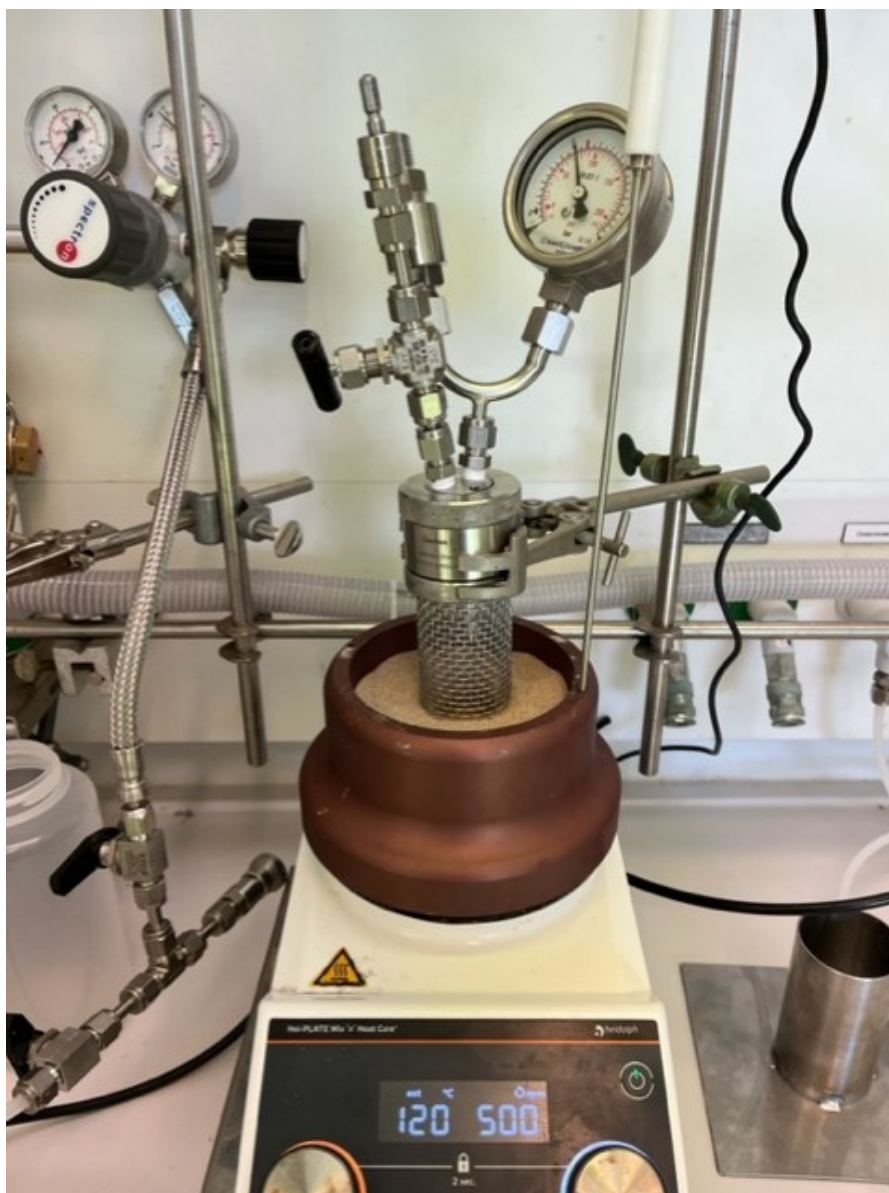
Figure 6.42: Autoclave used for boron radical activation reactions.
