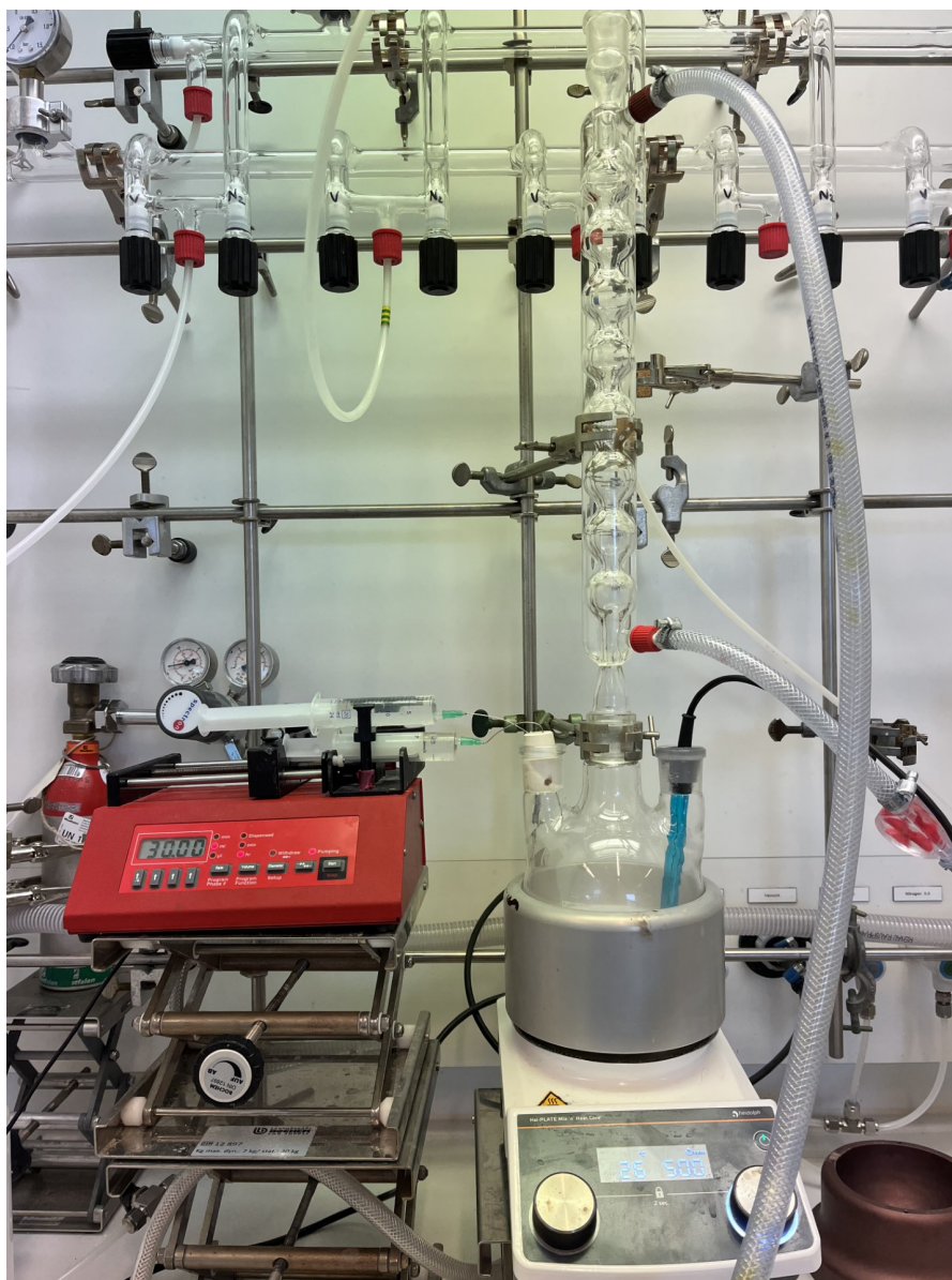
Figure 6.40: Fed-batch hydrogen release system through acid addition by syringe pump.
