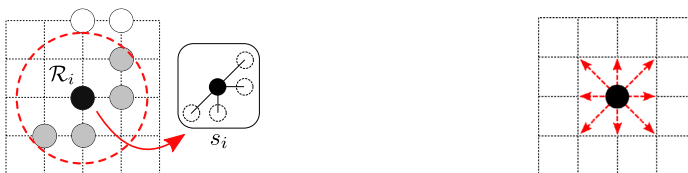
(a) Example of a local state s_i \in \mathcal{S} of a robot \mathcal{R}_i . The robot is shown in black and its neighbors within sensing range are shown in gray. It is assumed that a robot can always sense neighbors in the 8 grid points that surround it.
