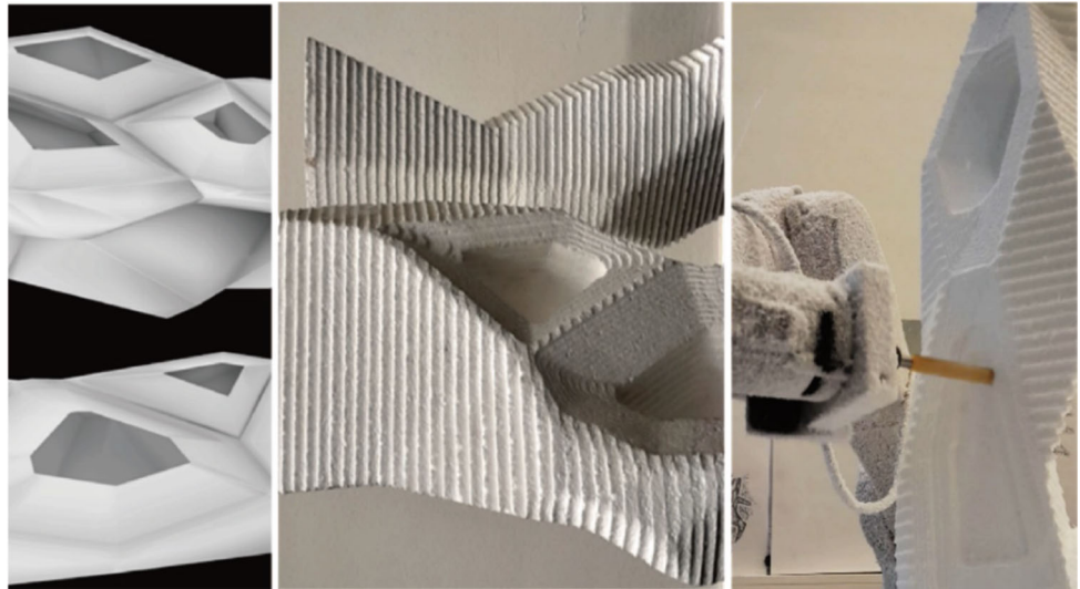
Fig. 4 Voronoi-based component design (left) and prototype (middle) milled by robot (right) from expanded polystyrene (EPS) (cited by RB Lab, TU Delft)
