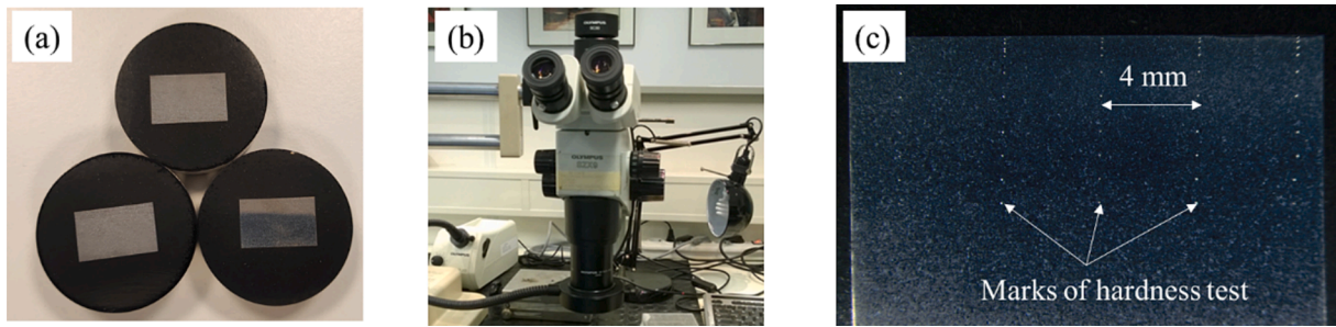
Fig. 3. Rail specimens and test methods. (a) rail specimens; (b) LOM; (c) micro-hardness test with remaining indentation marks in the specimen.
