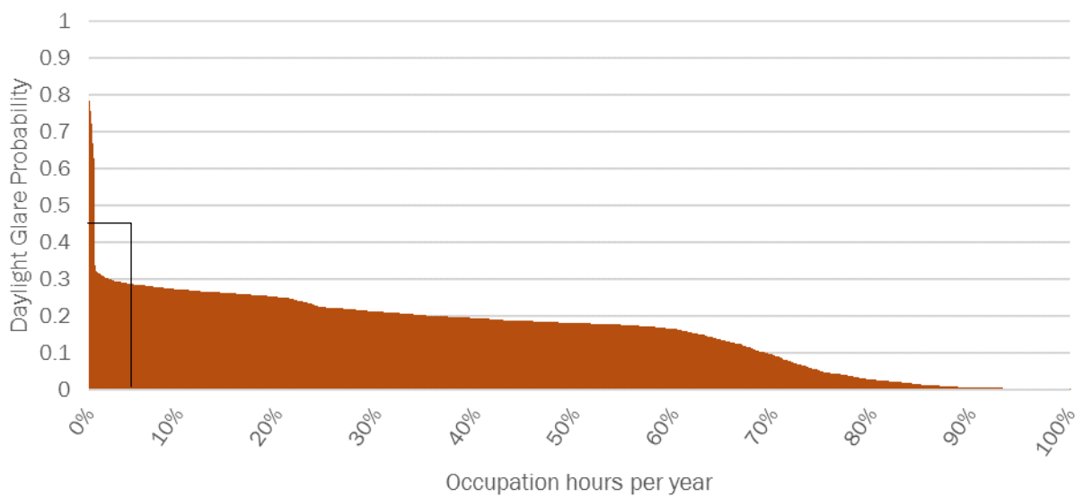
Daylight Glare Probability during a percentage of the occupation hours per year
