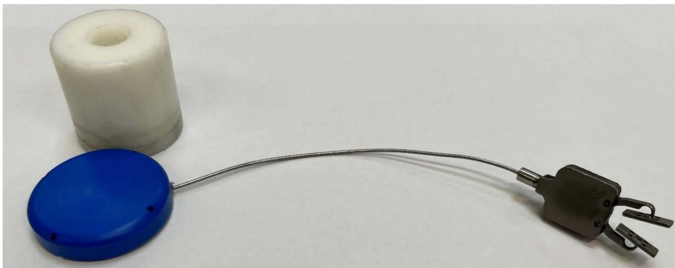
Fig. 10. Manufactured prototype of the implant device used in the experimental setup, and the external magnets that can be utilized to actuate the prototype.
