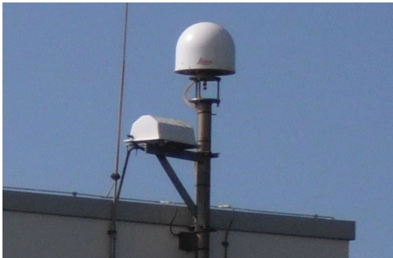
Fig. 20. GNSS station at IJmuiden, the Netherlands, with a co-located active radar transponder. Hereby, GNSS measurements and PSI measurements can be connected in the same geodetic datum. The GNSS receiver is placed within the round dome, whereas the radar transponder is contained within the white box.
