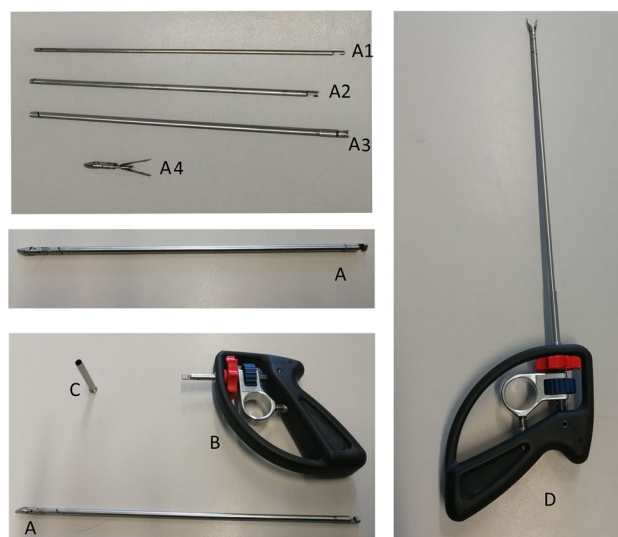
Fig. 5 Assembly and disassembly of the detachable multi-DOF grasper. Top left, the shaft contains the inner rod (A1) and the tubes (A2, A3), and at the end is the tip with sliders (A4). Middle left, the assembled shaft. Bottom left, the shaft (A) and handle (B) are connected and secured by sliding the coupling tube (C) over the connection
