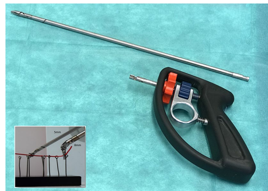
Fig. 8 SATA grasper handle detached from shaft assembly. Window image: 5 mm and 8 mm SATA instruments in action during a wire chasing training task
