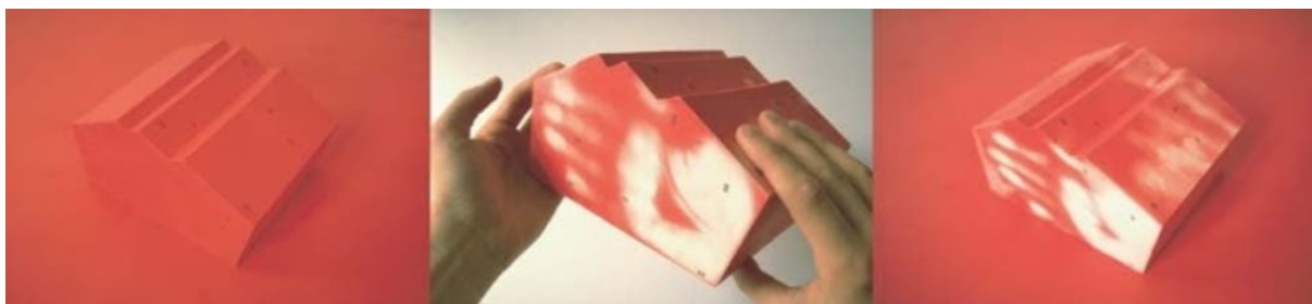
Figure 4.5 Example of thermochromic material. Note. From Addington & Schodek (2005).
