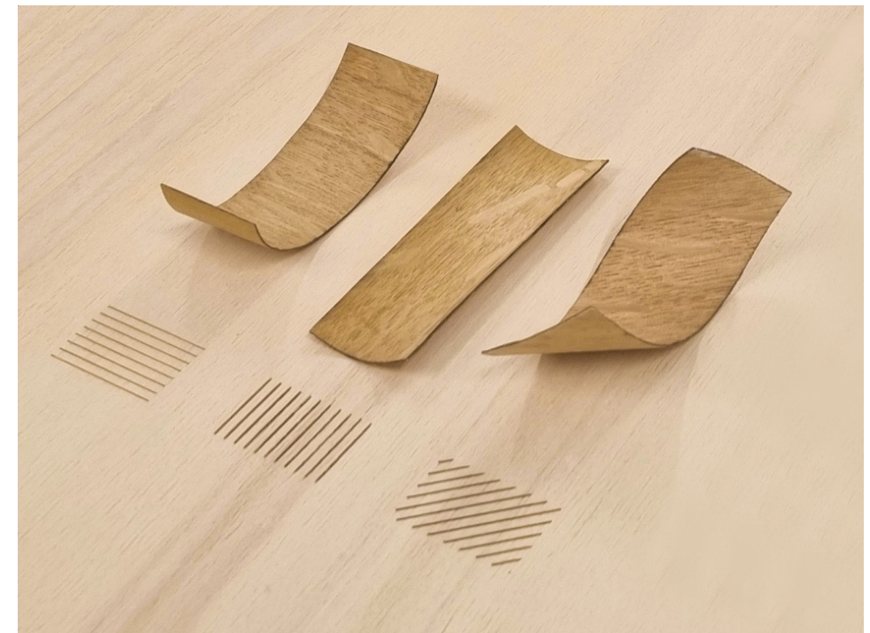
Fig 4. Fiber directions and resulting curvature response
