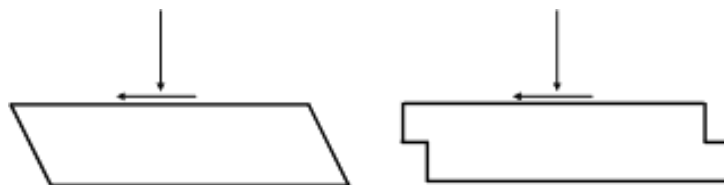
Figure 3.5: Schematic differences in the mode of shear failure direct simple shear test (L=Left) and direct shear test (R=Right)
