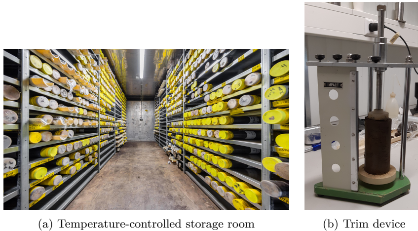
Figure 4.10: Preparing a triaxial sample
