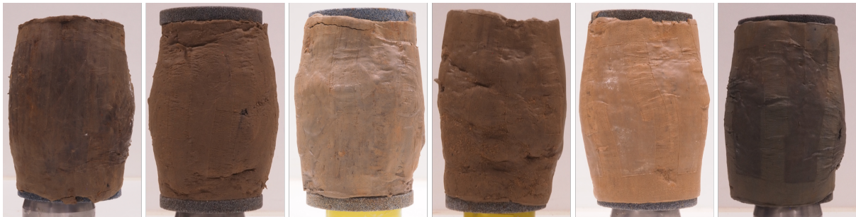
Figure 4.13: Overview of the failure mode corresponding to the driest specimen (L) to the fully saturated (R)
