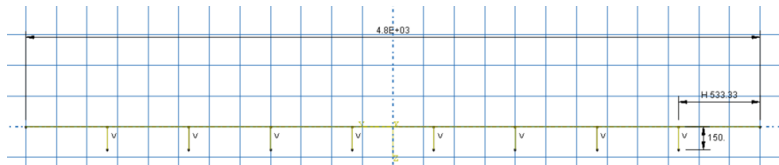
Figure 3:18 Configuration of the stiffened plate for validation of the model
