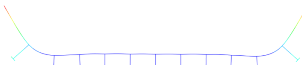
Figure 3:9 Dominant column-like buckling stiffeners side.
