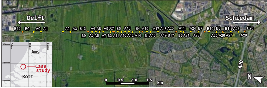
Figure 6.9: Overview of the Delft-Schiedam rail embankment and CPT surveys in the South Holland province.
