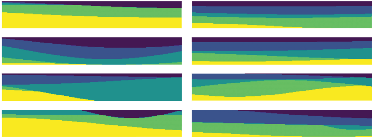
Figure 4.3: Synthetic models simulating subsoil layering variability with simple sub-horizontal layering, steep angles, irregular layers, indentations and complex geometries with lenses and old channels.
