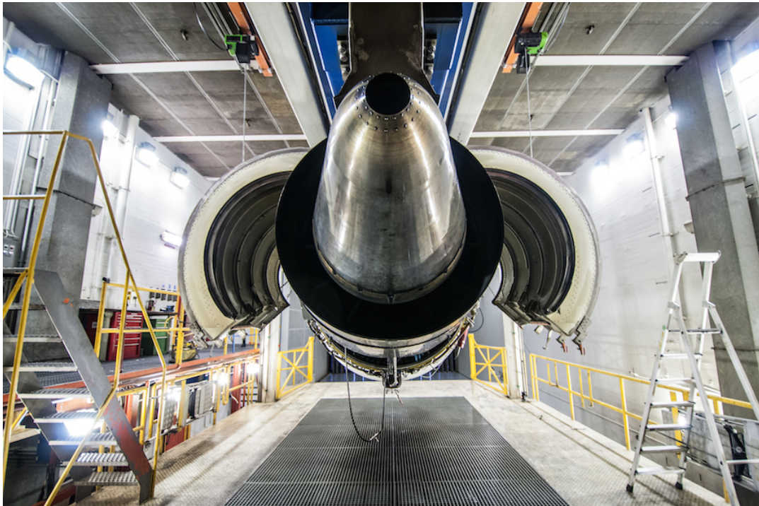
Figure 4.1: KLM E&M ES Test Cell Location With CF6 Engine, Image courtesy of KLM
