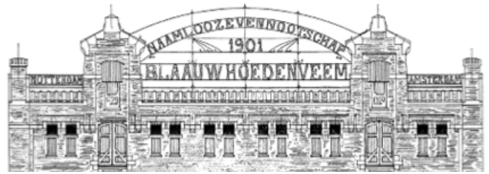
4.11 The original facade was characterised by the accents of the winch houses and the billboard.
