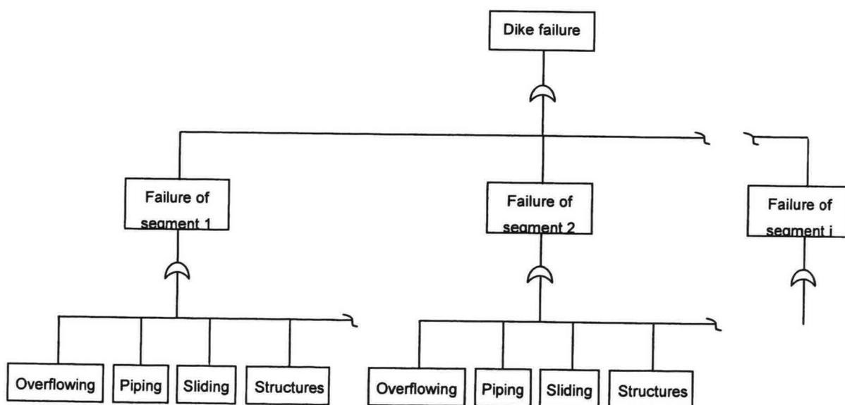
Figure 4.2 Fault tree of the dike
