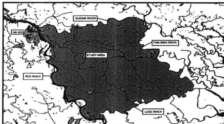
Figure 5.1 Potential inundation area in case of failure of the Duong River dike
