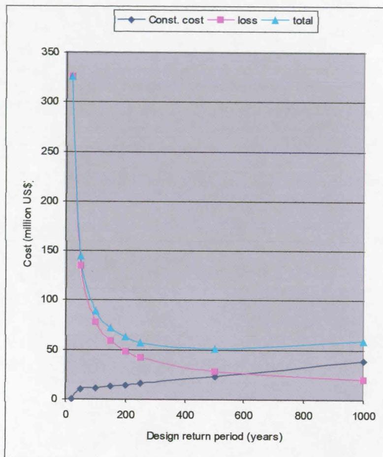
Figure 5.2 Determining the optimal height of the dike (upper boundary)
