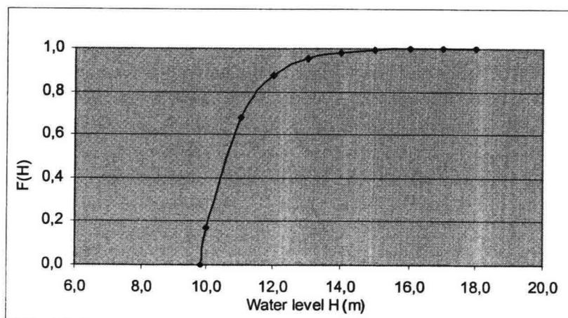
Figure 3.4 Distribution function of the highest water level at Thuong Cat
