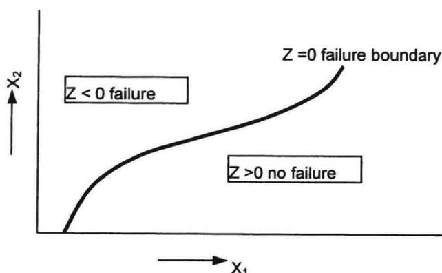
Figure 2.3 Definition of a failure boudary  $Z = 0$
