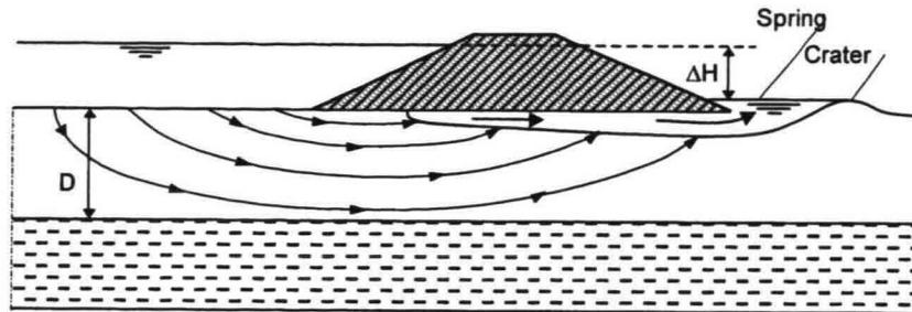
Figure 4.4 Mechanism of piping
