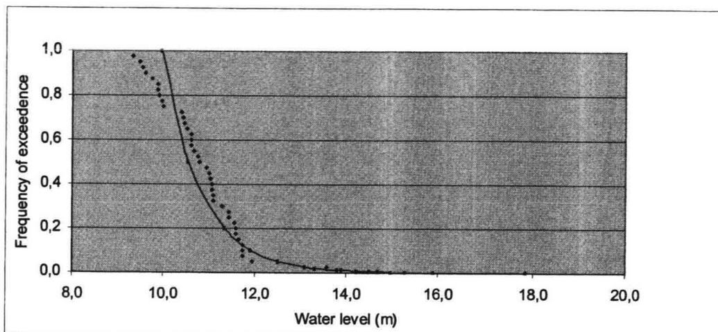
Figure 3.2 High water level frequency curve at Thuong Cat gauging station by using the Exponential distribution (method of moments)
