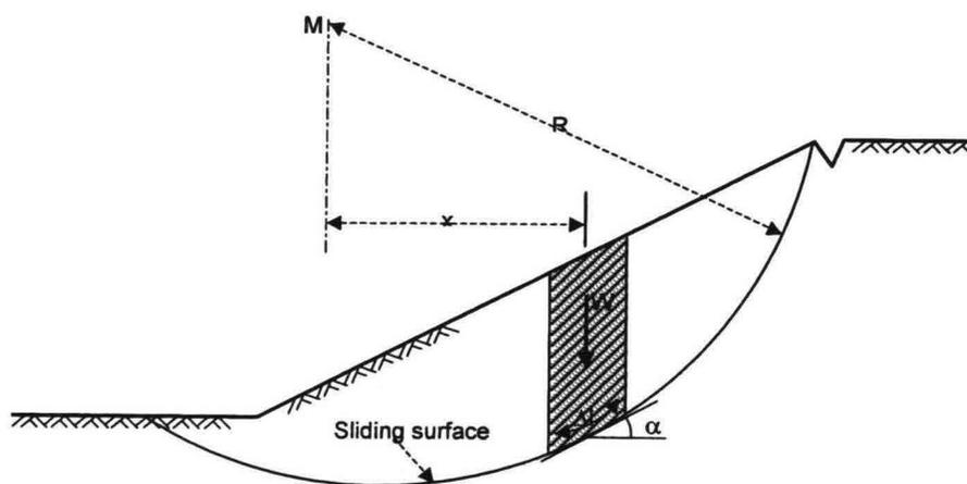
Figure 4.6 Mechanism of macro-instability
