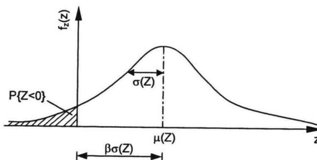
Figure 2.4 Probability density function of  $Z = R - S$ , showing the reliability index  $\beta$
