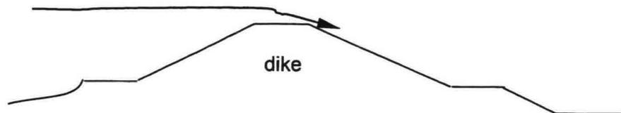
Figure 4.3 Mechanism of overflowing
