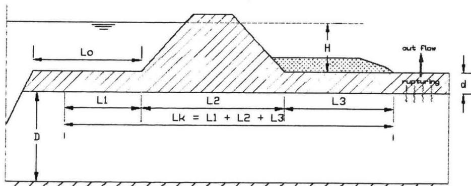
Figure 4.5 Determination of minimum seepage path length
