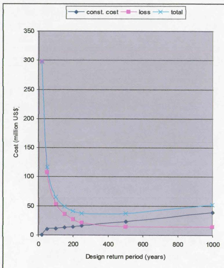
Figure 5.3 Determining the optimal height of the dike (lower boundary)
