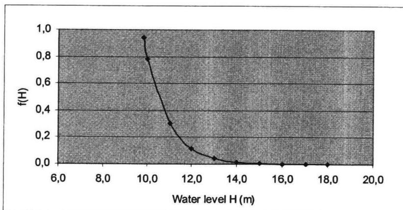
Figure 3.3 Probability density function of the highest water level at Thuong Cat
