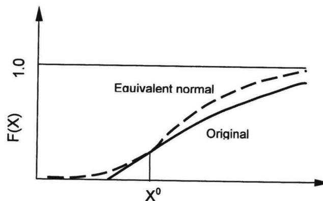
Figure 2.6 Replacing a non-normal distribution by a normal distribution
