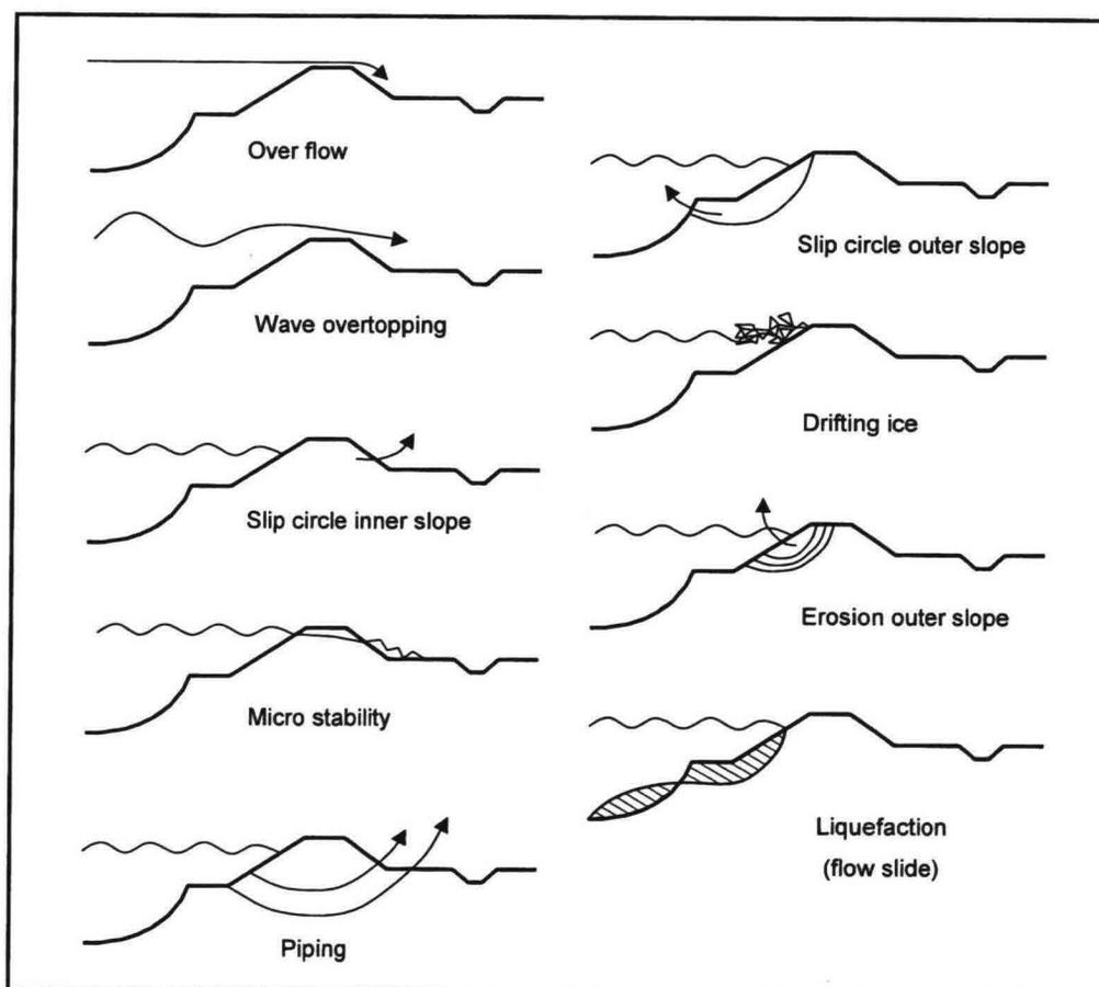
Figure 4.1 Failure mechanisms for dikes
