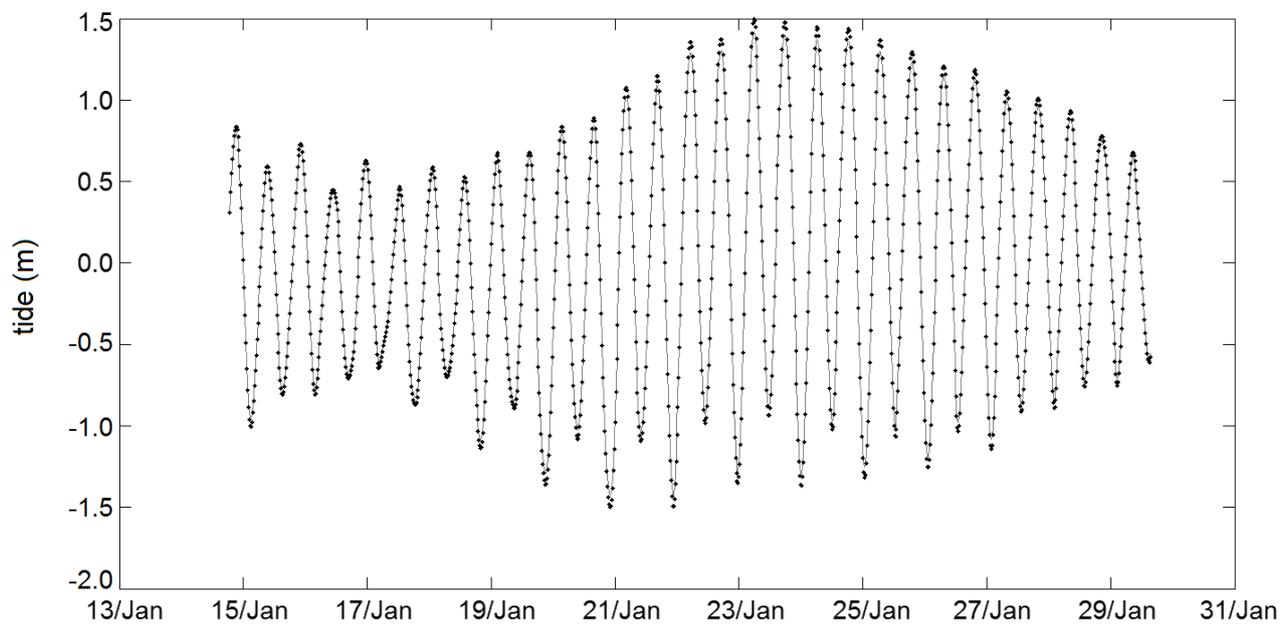
Figure 5 – Modelled water column (m) at station A compared to measured tides, from 14<sup>th</sup> to 29<sup>th</sup> of January 2008. Dots denote observations, and line denotes model result.
