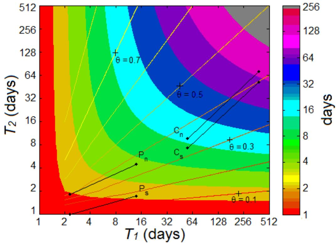
Figure 10 – The position of Caravelas (CA) and Peruípe (P) estuaries on the advection-diffusion diagram to indicate the relative contribution to the water renewal  $T_P$  by the advective ( $T_1$ ) and dispersive ( $T_2$ ) timescales using a logarithmic scale. Subscript (n) and (s) indicate neap and spring tide conditions.
