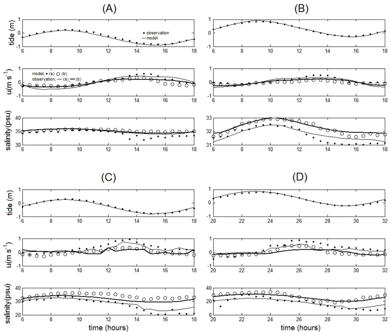
Figure 6 – Modelled tide (m), axial channel velocity  $u$  ( $\text{m s}^{-1}$ ) and salinity (psu) compared to measured time series at stations A, B, C, and D, during neap tides. Measurements and simulation represented at the surface and bottom layers. Skill values are synthesised in Table 4.
