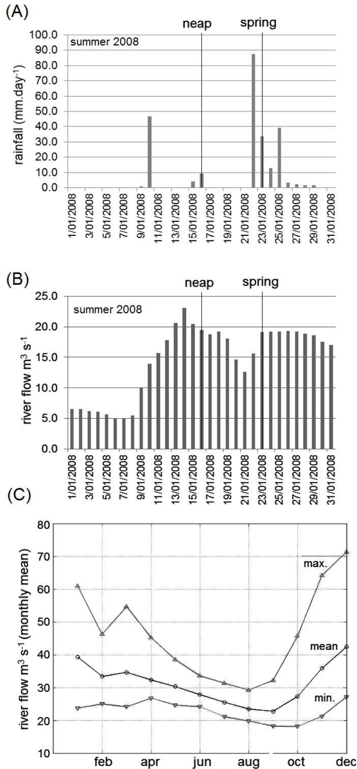
Figure 3 – Daily variation of the rainfall (A), and river discharge (B) during January (2008), observations were made at the gauge station *Helvécia* n° 55510000 (código 1739006) – National Agency of Waters. (C) Climatological estimate of the mean, minimum (min.) and maximum (max.) monthly river discharge using data from 1975 to 2008 (34 years of measured river flow) and corrected using the factor 1.6 to account for the entire drainage basin area of the *Peruípe* River.
