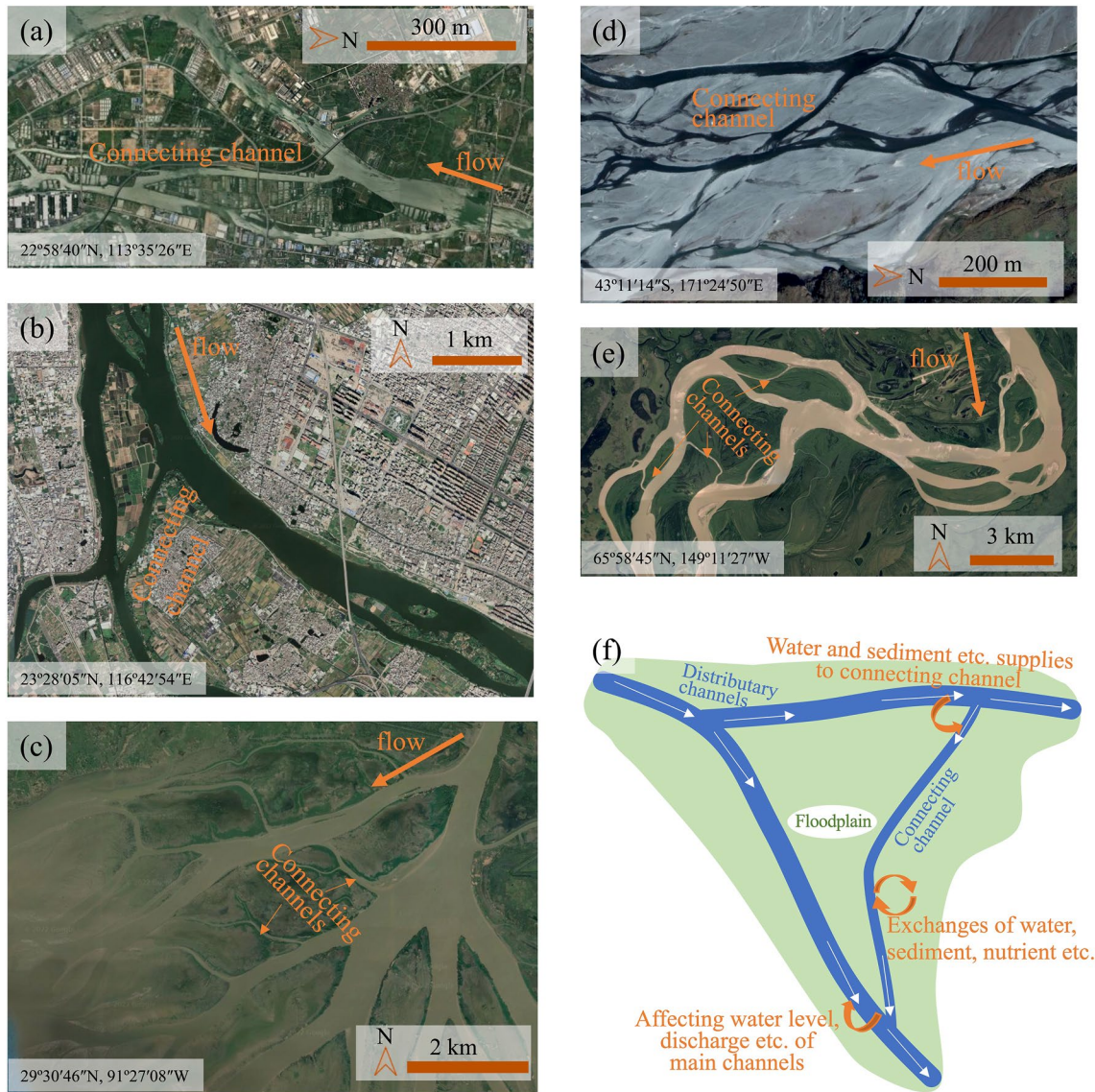
Figure 1. Examples of connecting channels in river deltas, braided rivers and anastomosing rivers: (a) the Dongjiang Delta (a subdelta of the Pearl River Delta) and (b) the Hanjiang Delta, in Guangdong, China, (c) the Wax Lake Delta, USA, (d) braided channels of the Wilberforce River, New Zealand, and (e) anastomosing channels of the Yukon River, USA. (f) A schematic showing the interactions between rivers and their floodplain through the floodplain connecting channels. Satellite images are from Google Earth ( https://earth.google.com/ ).
