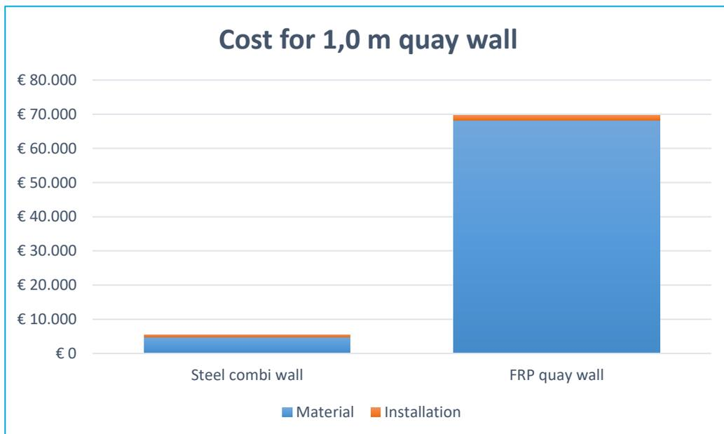
Figure 39: The cost for 1,0 m quay wall for both materials
