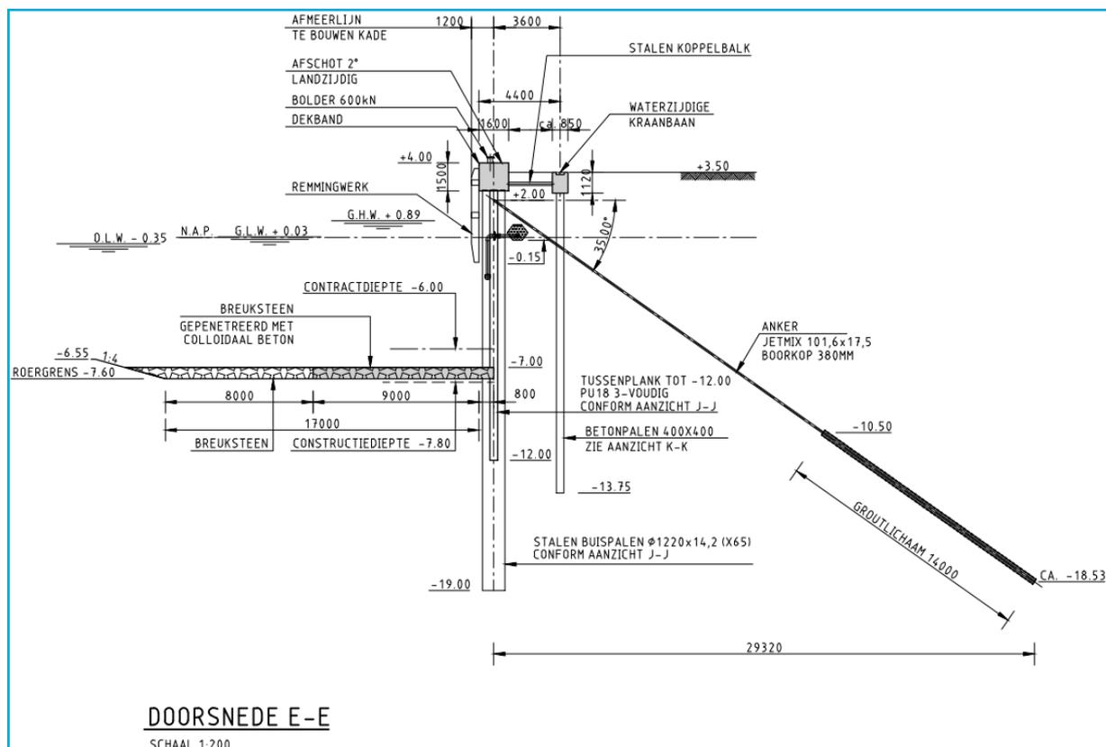
Figure 2: Cross section of the design of the quay wall
