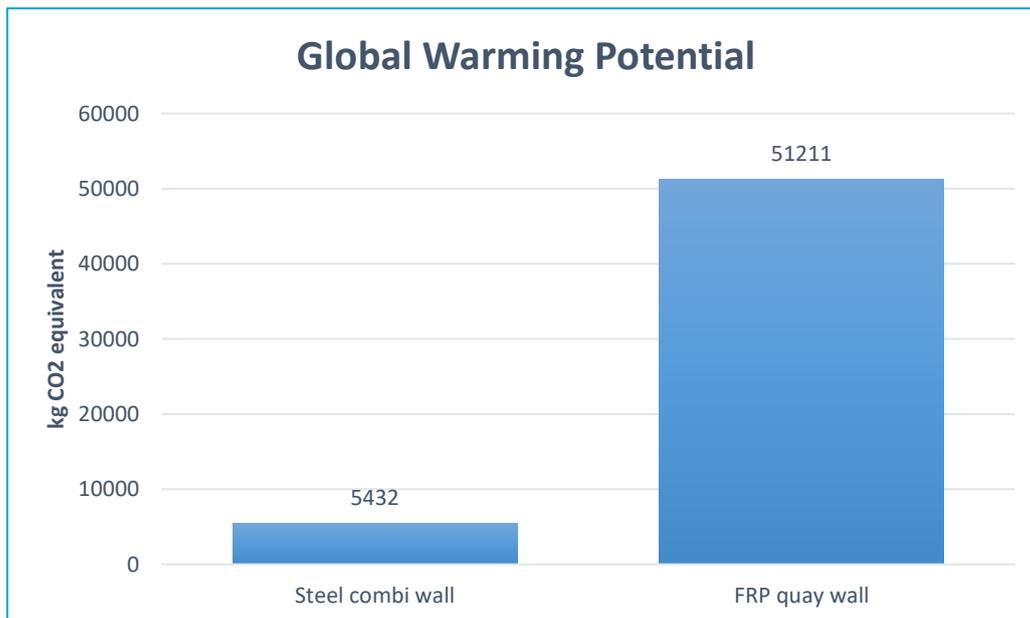
Figure 35: Global Warming Potential for the phase 'manufacturing elements'
