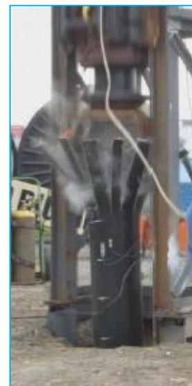
Figure 32: Splitted pile head [ACE, 2012]
