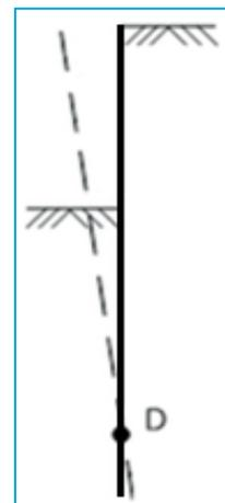
Figure 6: Cantilever sheet pile
