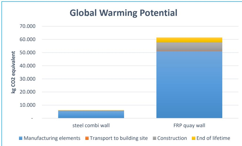
Figure 34: Global Warming Potential of the quay walls
