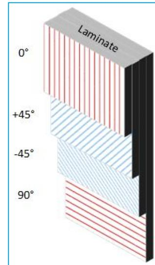
Figure 16: Applied fibre directions
