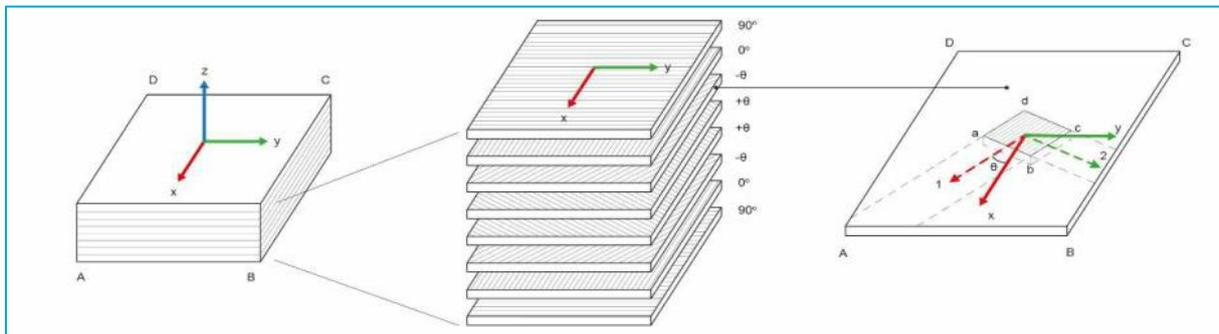
Figure 17: Reference axes of a oriented lamella  $abcd$  (1,2) with respect to global laminate axes  $(x,y)$  (plate  $ABCD$ ) [CUR96, 2016]
