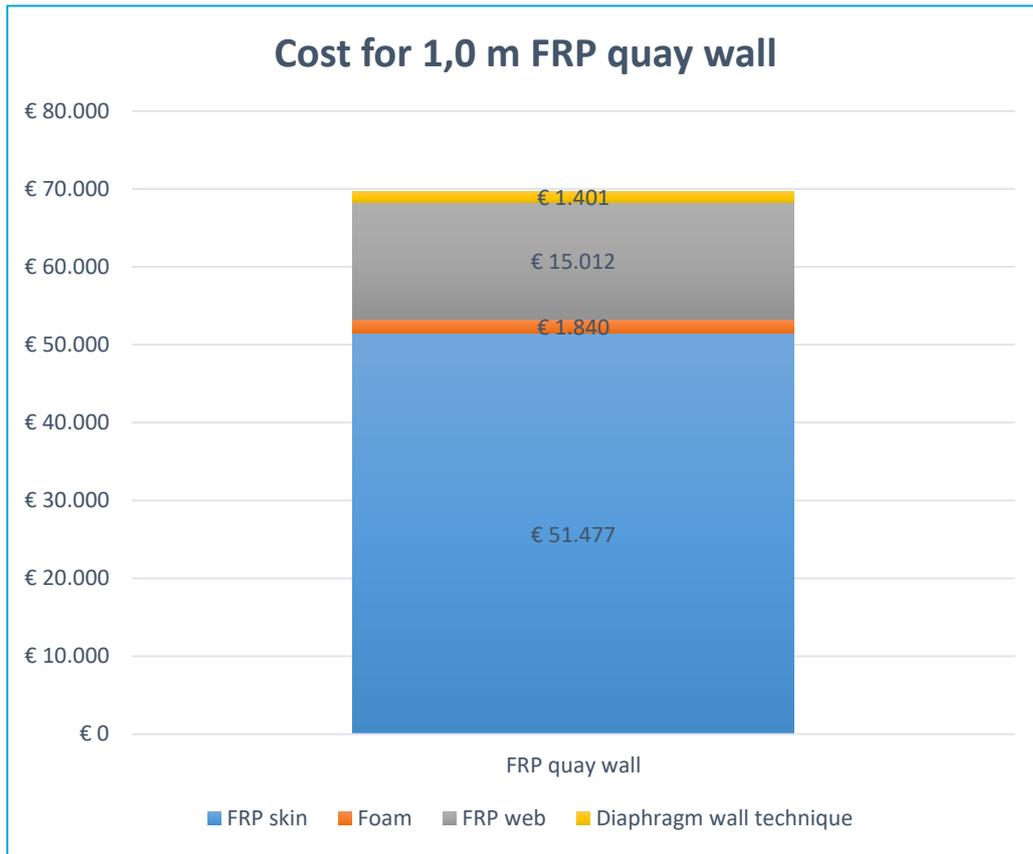
Figure 38: Cost estimation of 1,0 m FRP quay wall
