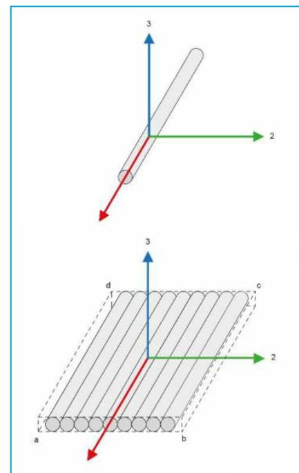
Figure 15: Reference axes of a fibre and lamella [CUR96, 2016]
