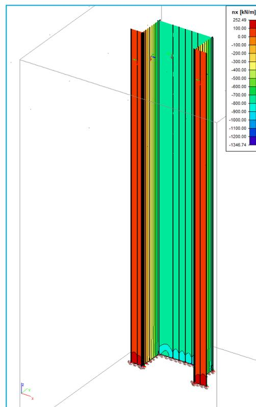
Figure 25:  $N_x$  distribution in the SLS
