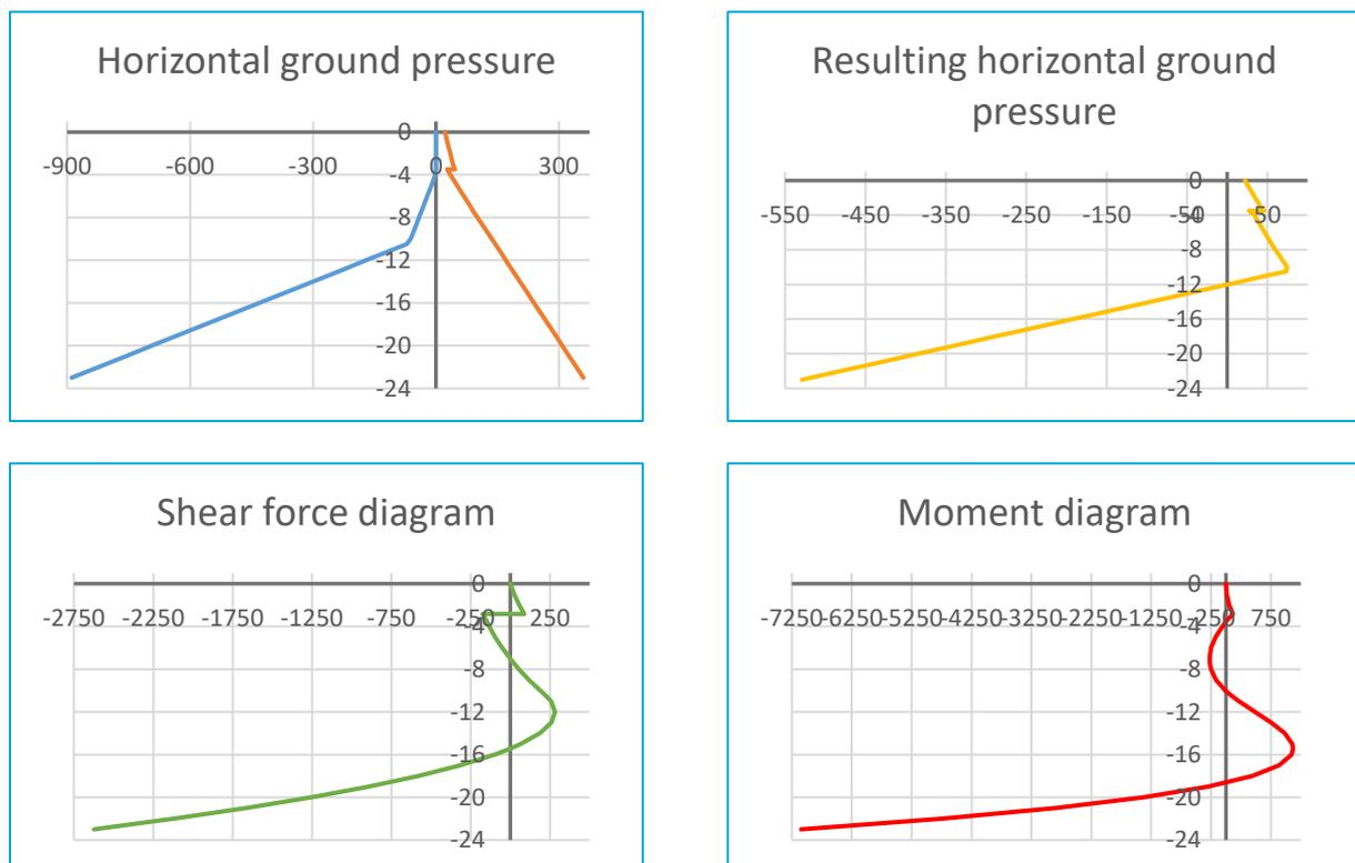
Figure 9: Diagrams belonging to the anchored sheet pile quay wall
