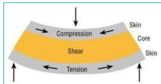
Figure 4: Sandwich construction in bending [Cripps, 2016]
