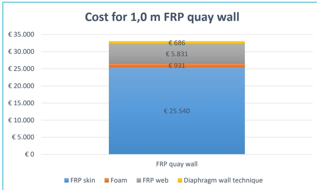
Figure 41: Cost for 1 meter FRP quay wall with dimensions corresponding to design 1
