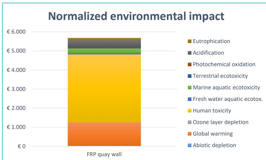
Figure 40: Normalized environmental impact for an FRP quay wall with dimensions corresponding to design 1
