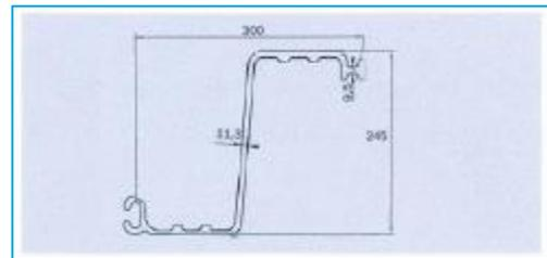
Figure 30: Example of a connection profile [Bergschenhoek, 2016]
