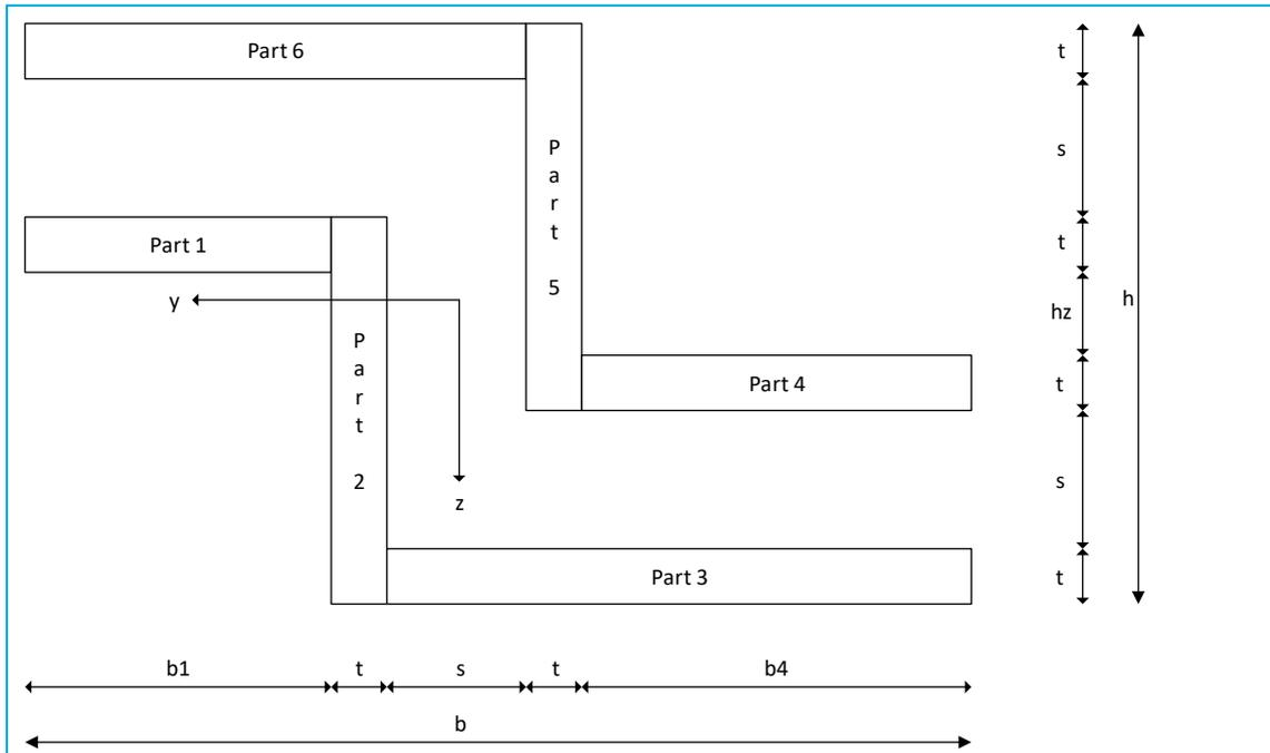
Figure 14: Schematization of the cross section
