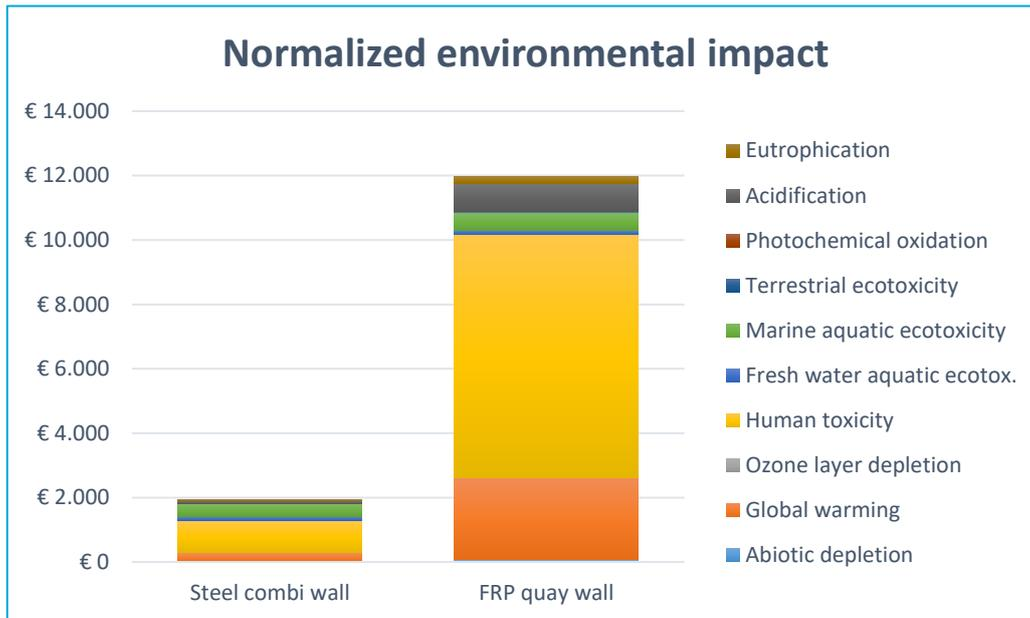
Figure 36: Normalized environmental impact for both types of quay walls
