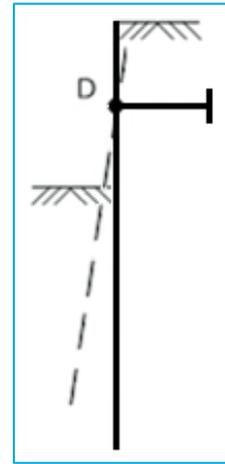
Figure 7: Anchored sheet pile
