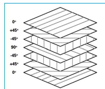
Figure 5: Example of a stacking order [Cripps, 2016]
