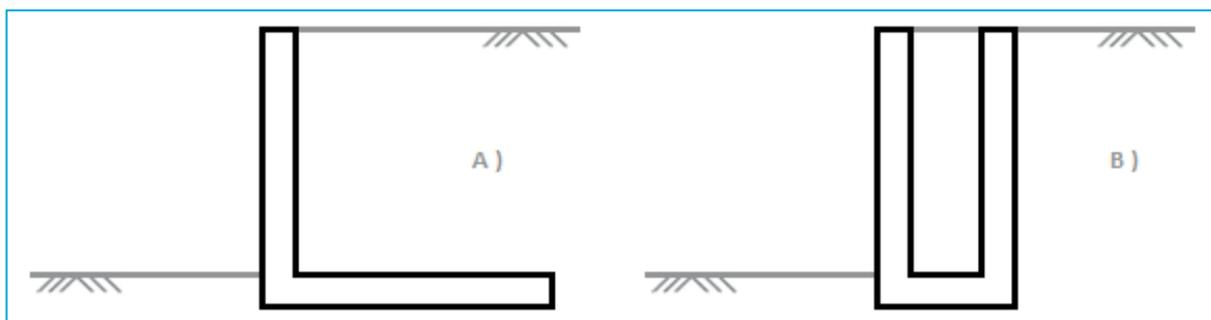
Figure 8: A) representation of an L-wall; B) representation of a caisson
