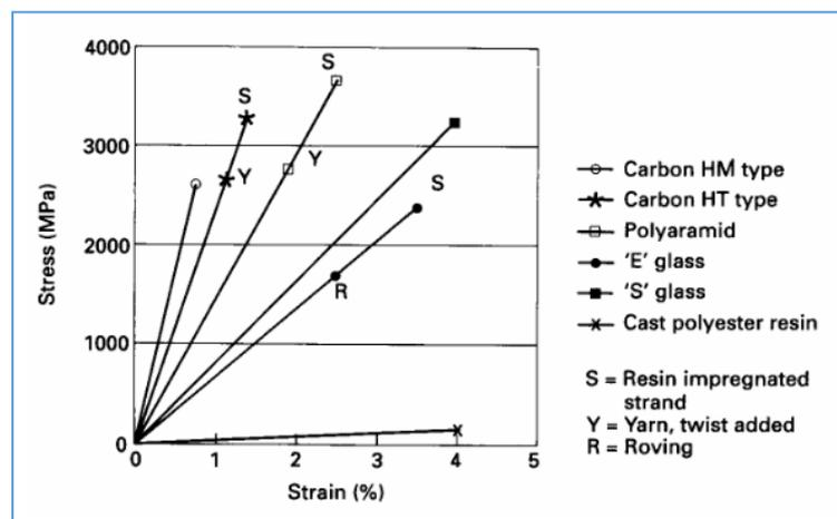
Figure 3: Stress-strain curves of reinforced fibres
