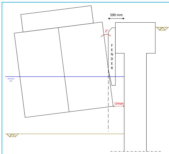
Figure 11: Determination of the maximum deflection. Not to scale
