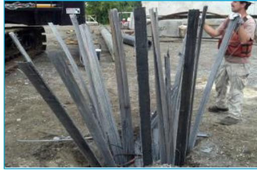
Figure 33: Damaged pile head after removal of the hammer [ACE, 2012]
