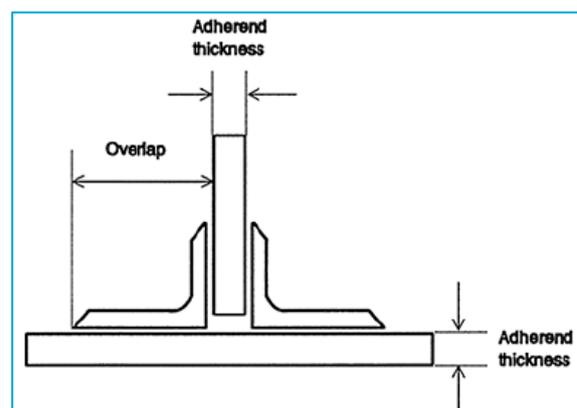
Figure 29: Representation of a T-joint
