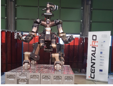
Fig. 7. The wheeled quadrupedal centaur-like robot CENTAURO.
