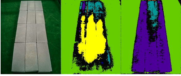
Fig. 4. Effect of data augmentation techniques. From left to right: an image from an RGB camera, prediction without, and with brightness and contrast adjustments.
