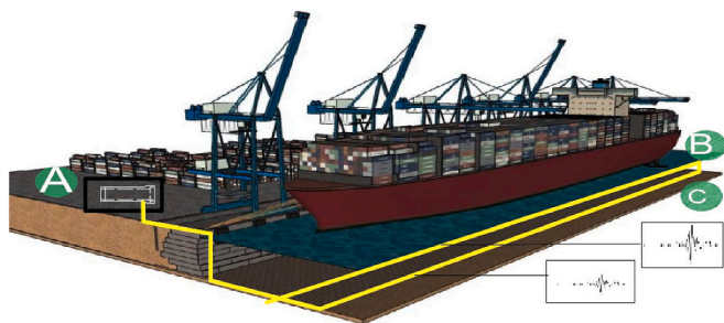
Fig. 4. Potential setup for monitoring the water-mud interface. Here A is an observation station with a DAS interrogator onshore, B is the line suspended in water in this particular situation, and C is a line in (fluid) mud.
