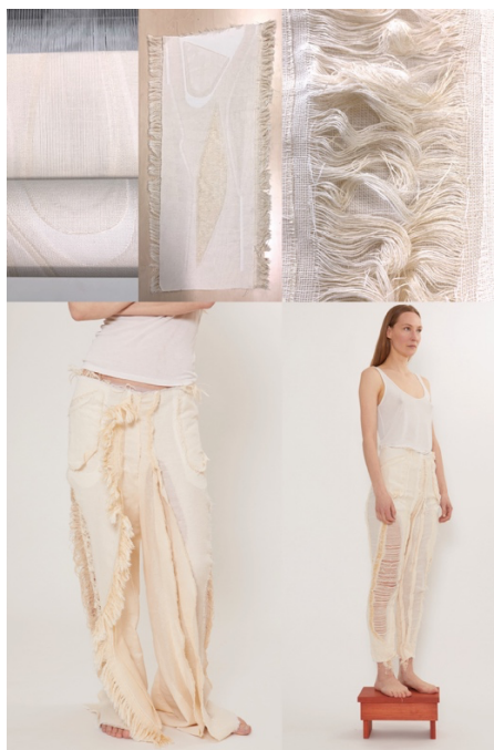
Figure 4: Top left: Trousers on loom. Top middle: Loomstate textile. Top right: Detail of yarn behaviour after cutting. Bottom left: unsprung trousers. Bottom right: The same trousers shrunk in dryer. Darker cream yarn in weft direction (most easily seen in third image) is NSK heat reactive yarn, lighter cream is cotton weft and warp. This colour difference reveals the variety of layer composition in the resulting loom state textile that causes complex behaviours to emerge once 3D form is released through cutting and heating.
