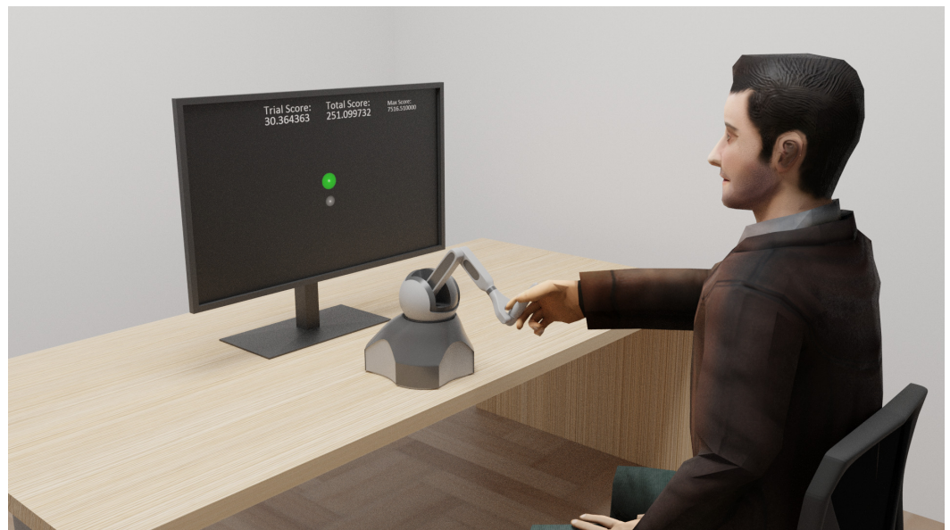
Figure 1. Experimental setup. The robot was aligned with the center of the screen. All subjects were requested to keep the center of their chest in line with the robot and the center of the screen.
