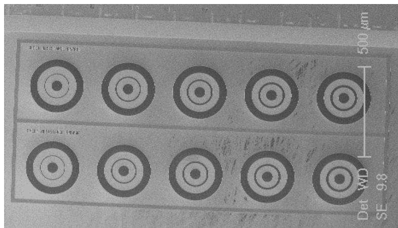
Figure 2.8: SEM images of test structures to calculate the sheet resistance of PureB.
