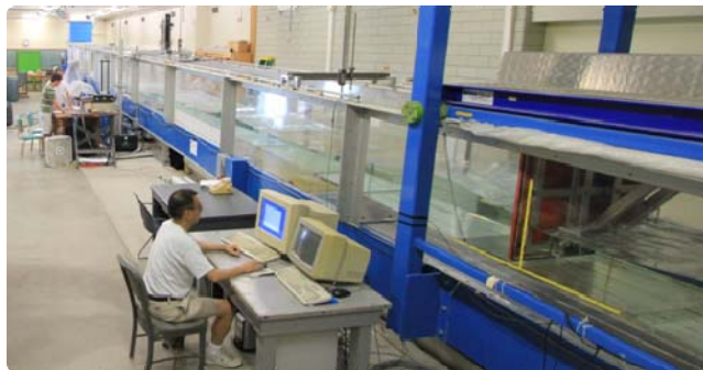
Figure 2: Wave flume and wave generator.
