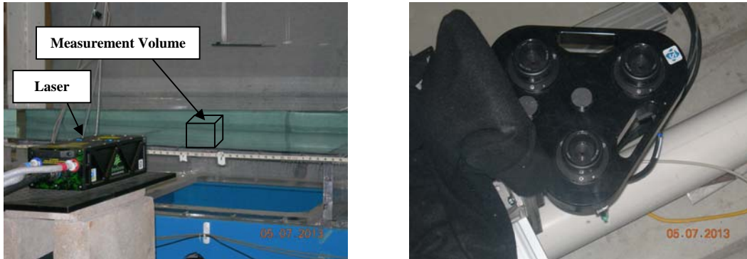
Figure 3: Laser and measurement volume (left), and V3V camera (right) looking at the measurement volume from underneath the flume.
