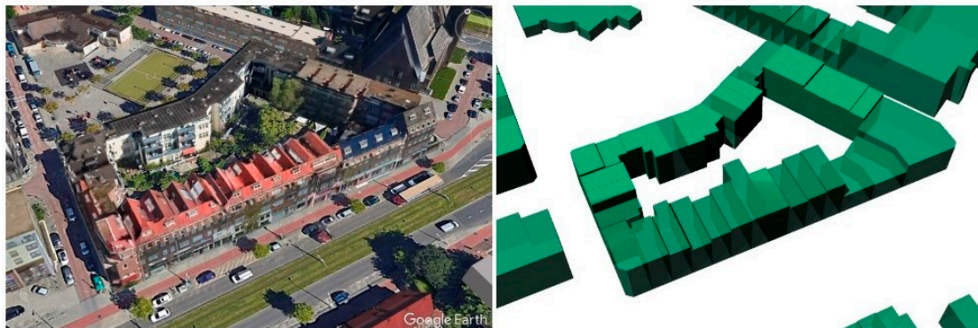
Figure 2. Satellite image from Google Earth of the Hilleshuis neighbourhood (left). “Level of Detail 1” (LOD1) model of multiple adjacent buildings (right).
