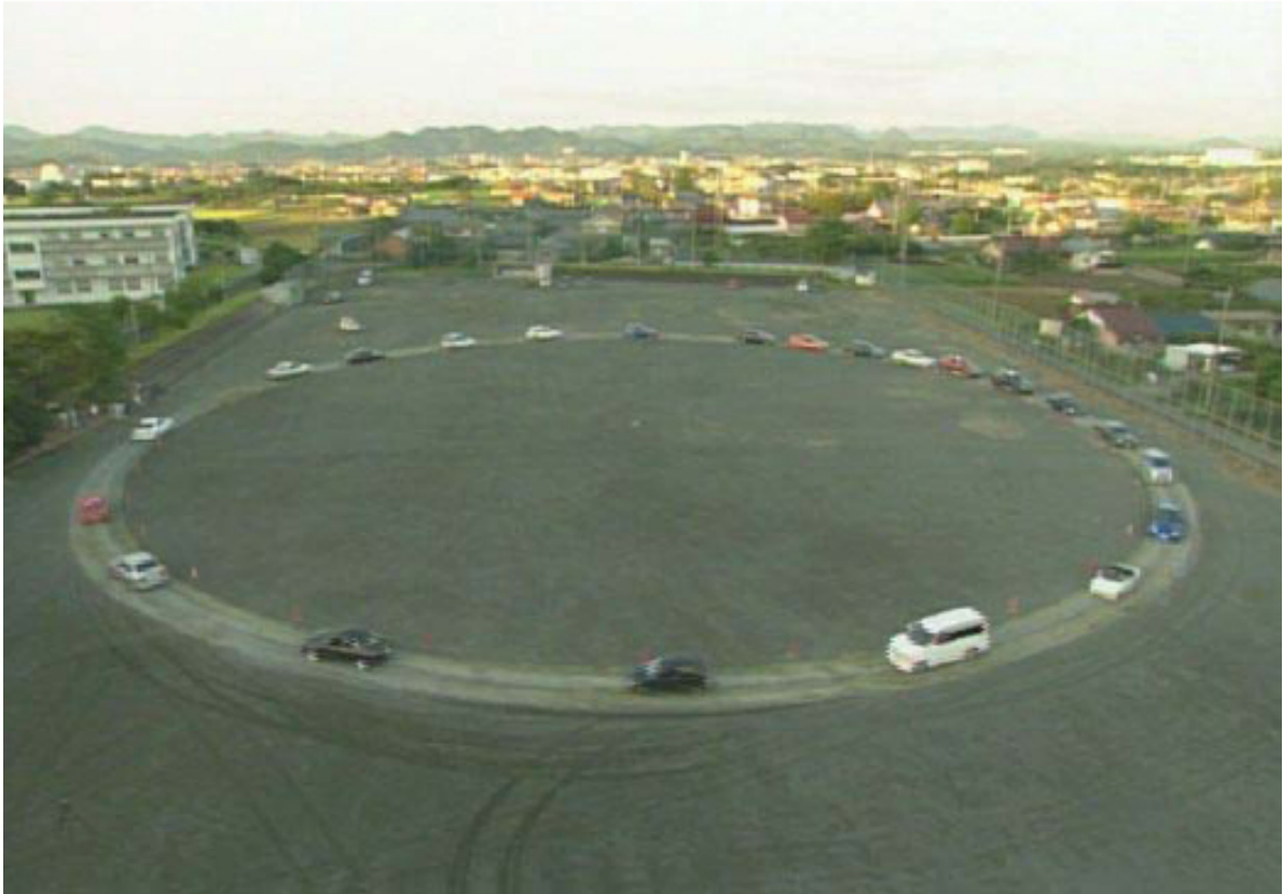
Figure 1-1: A snapshot of the experiment on a circular road [1]. In this case, the circumference is 230m, and the number of vehicles is 22.
