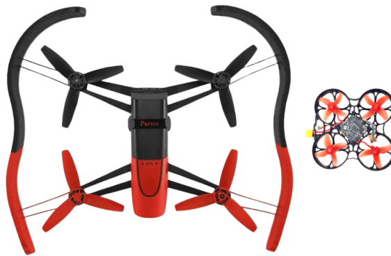
Figure A.1: The Eachine Trashcan has the same size as a propeller of the Parrot Bebop.
