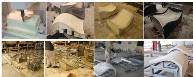
Fig: **Foam & Steel Formwork** (Ock, 2021)
