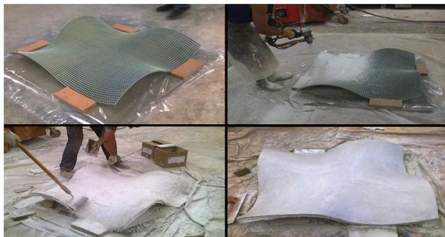
Fig: **AM Formwork** (Vergara et al., 2017)
