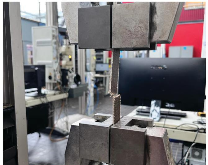
**Table - C 464 - Ultimate Tensile Properties Before & After Reshaping**
