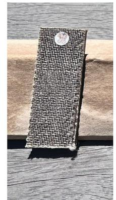
The fraying & fade might be a result of the thin PLA layers (70:30 mass ratio) wearing away, leaving the flax fibers unprotected.
