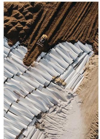
Fig 7: GFRP Blades buried in landfill, 2020 Wyoming, USA
