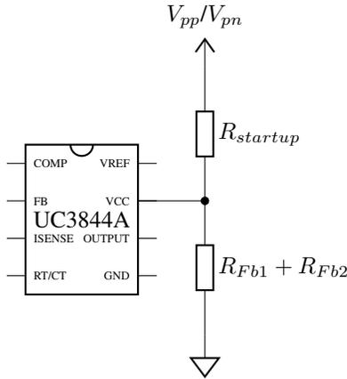
Fig. 5. Startup circuit for the flyback transformer.
