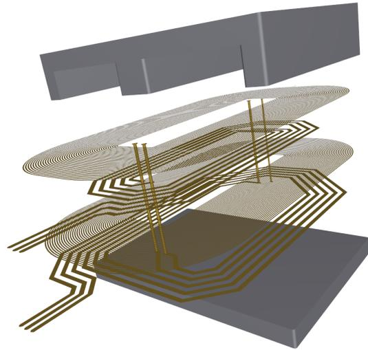
Fig. 2. Exploded 3D figure of design 1 for the planar flyback transformer.
