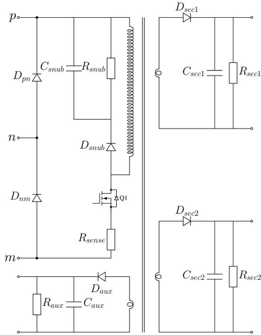
Fig. 1. Schematic of the flyback transformer.
