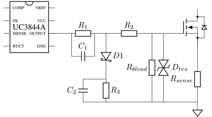
Fig. 6. Circuit used for level shifting the gate signal.
