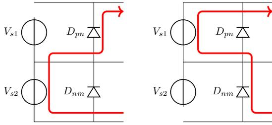
Fig. 7. Figures illustrate the current flow by a red arrow when one of the poles is out of service. Left: The converter  $V_{s1}$  is out of service; Right: The converter  $V_{s2}$  is out of service.
