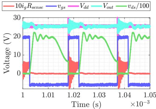
Fig. 9. Results for the converter operating at 1260 V input with 1.25 A output current.
