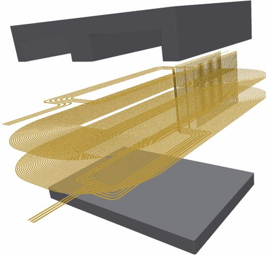
Fig. 3. Exploded 3D figure of design 2 for the planar flyback transformer.
