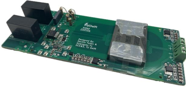
Fig. 8. Designed flyback converter.
