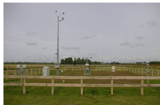
(b) Lay-out of a weather station.
